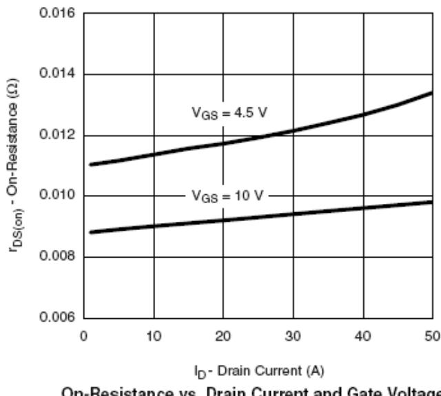
On-Resistance vs. Drain Current and Gate Voltage
