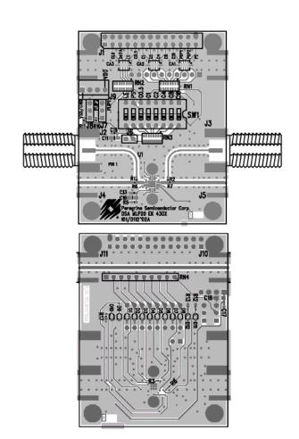
Figure 5. Evaluation Board Schematic
