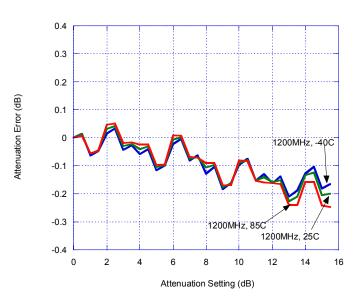
Note: Positive attenuation error indicates higher attenuation than target value
