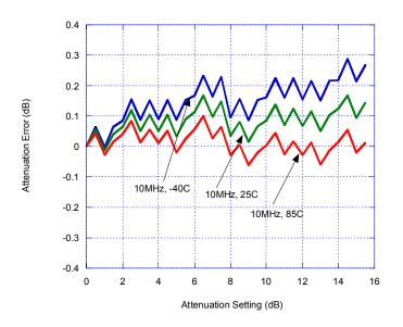
Figure 15. Attenuation Error Vs. Attenuation Setting
