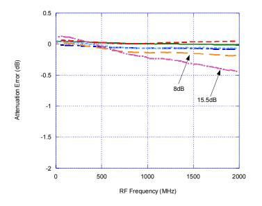
Figure 11. Attenuation Error Vs. Attenuation Setting
