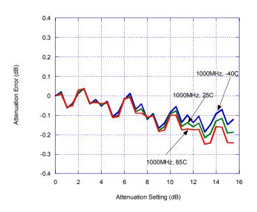
Figure 17. Attenuation Error Vs. Attenuation Setting
