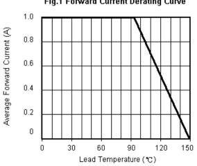
Fig.1 Forward Current Derating Curve
