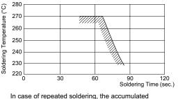
soldering time must be within the range shown above.
