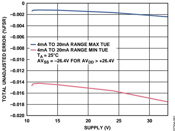
Figure 45. Total Unadjusted Error vs.  $AV_{DD}$ , Internal  $R_{SET}$
