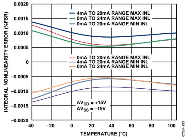
Figure 35. Integral Nonlinearity vs. Temperature, External RSET
