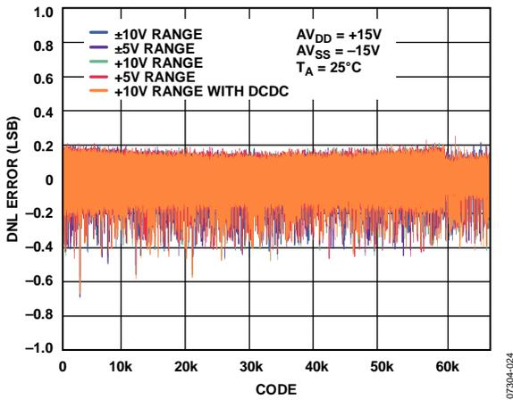
Figure 9. Differential Nonlinearity Error vs. DAC Code
