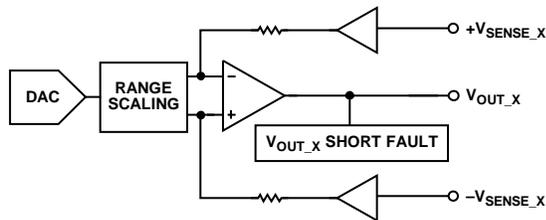
Figure 71. Voltage Output
