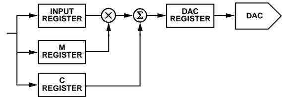
Figure 76. Digital Offset and Gain control
