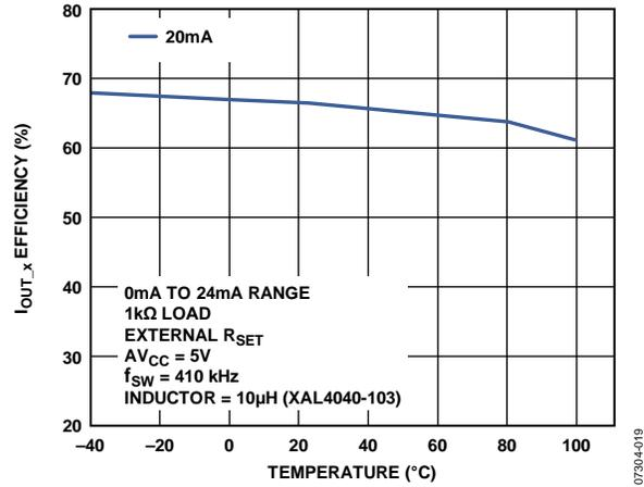
Figure 57. Output Efficiency vs. Temperature (See Figure 78)
