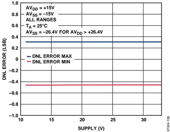
Figure 20. Differential Nonlinearity Error vs.  $AV_{DD}/AV_{SS}$
