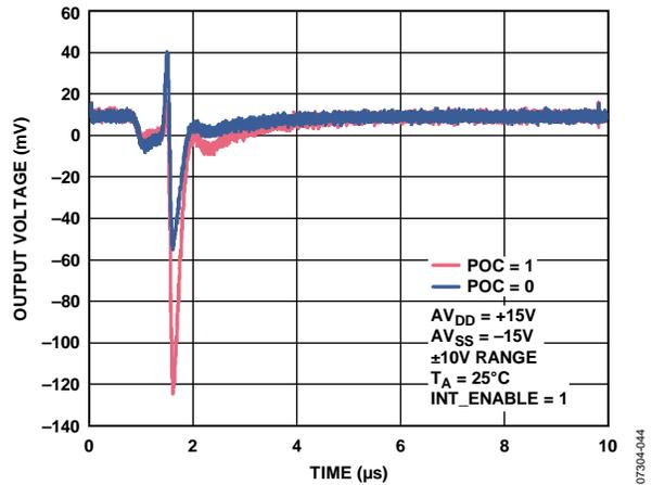
Figure 29.  $V_{OUT\_x}$  vs. Time on Output Enable
