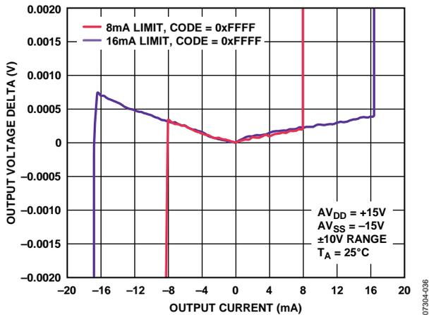
Figure 22. Source and Sink Capability of Output Amplifier
