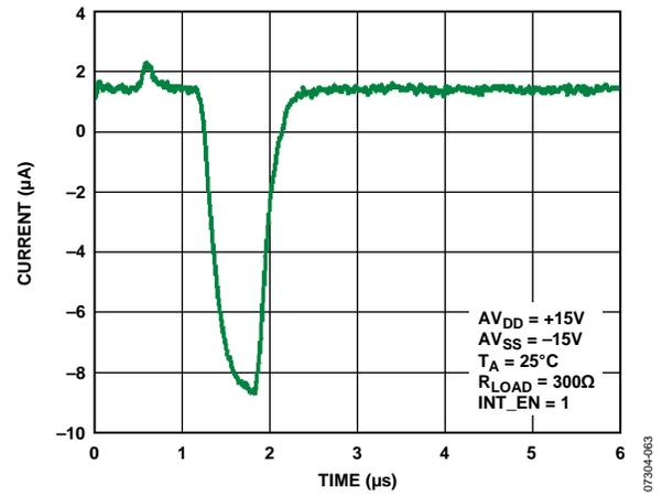
Figure 47. Output Current vs. Time on Output Enable
