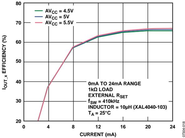
Figure 56. Output Efficiency vs. Output Current (See Figure 78)
