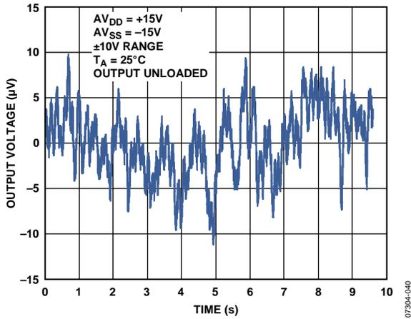
Figure 26. Peak-to-Peak Noise (0.1 Hz to 10 Hz Bandwidth)
