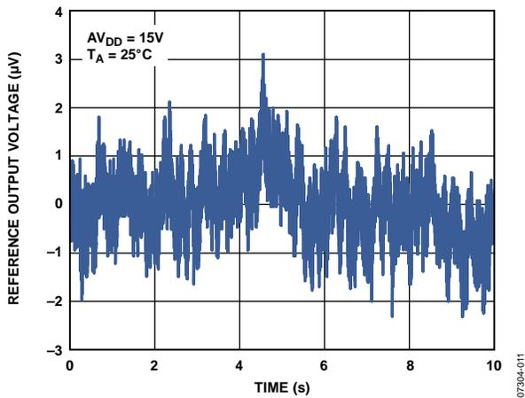
Figure 60. REFOUT Output Noise (0.1 Hz to 10 Hz Bandwidth)
