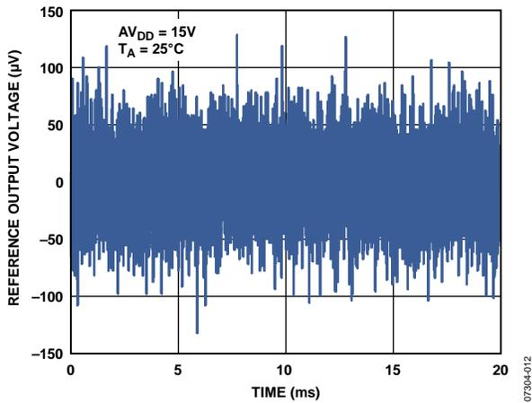
Figure 61. REFOUT Output Noise (100 kHz Bandwidth)
