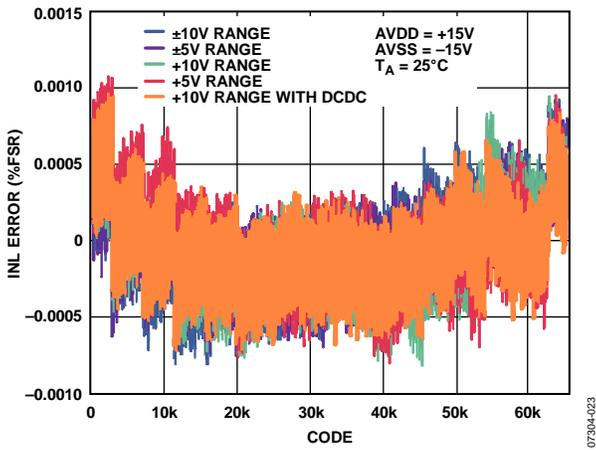
Figure 8. Integral Nonlinearity Error vs. DAC Code
