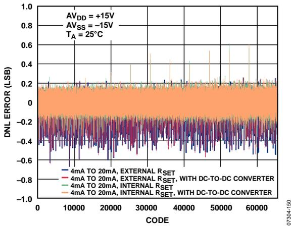
Figure 32. Differential Nonlinearity vs. Code
