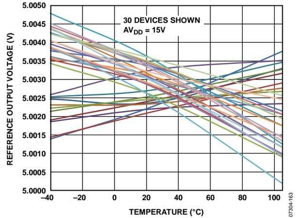
Figure 62. REFOUT vs. Temperature (When the AD5755 is soldered onto a PCB, the reference shifts due to thermal shock on the package. The average output voltage shift is  $-4$  mV. Measurement of these parts after seven days shows that the outputs typically shift back 2 mV toward their initial values. This second shift is due to the relaxation of stress incurred during soldering.)
