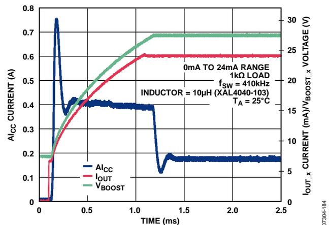
Figure 80. AI<sub>CC</sub> Current vs. Time for 24 mA Step Through 1 k $\Omega$  Load with Internal Compensation Resistor
