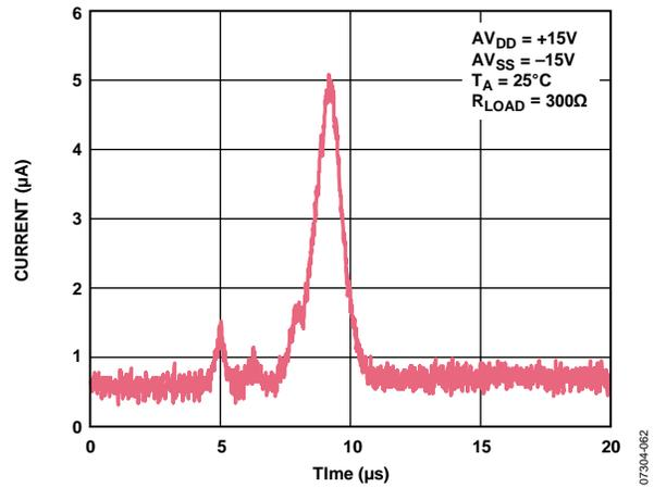
Figure 46. Output Current vs. Time on Power-Up
