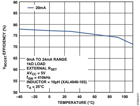
Figure 55. Efficiency at  $V_{BOOST\_X}$  vs. Temperature (See Figure 78)
