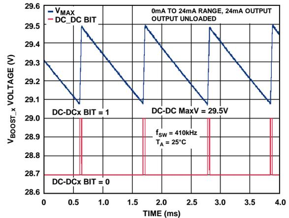
Figure 79. Operation on Reaching V<sub>MAX</sub>
