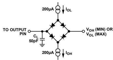
Figure 6. Load Circuit for SDO Timing Diagram
