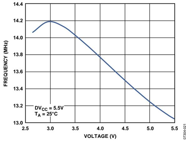
Figure 69. Internal Oscillator Frequency vs.  $DV_{CC}$  Supply Voltage
