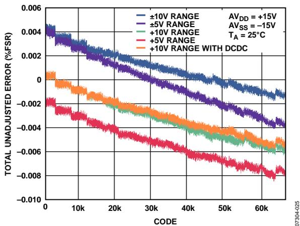
Figure 10. Total Unadjusted Error vs. DAC Code
