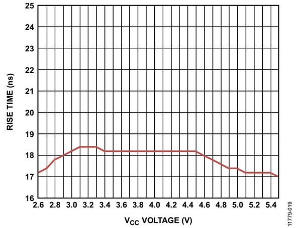
Figure 19.  $\overline{RESET}$  Push-Pull Rise Time vs.  $V_{CC}$  Voltage
