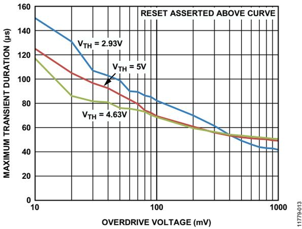
Figure 13. Maximum  $V_{CC}$  Transient Duration vs.  $\overline{RESET}$  Threshold Overdrive
