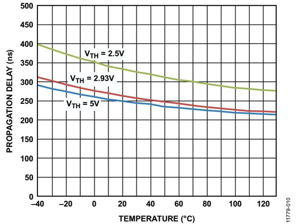
Figure 10. Manual Reset to Reset Propagation Delay vs. Temperature
