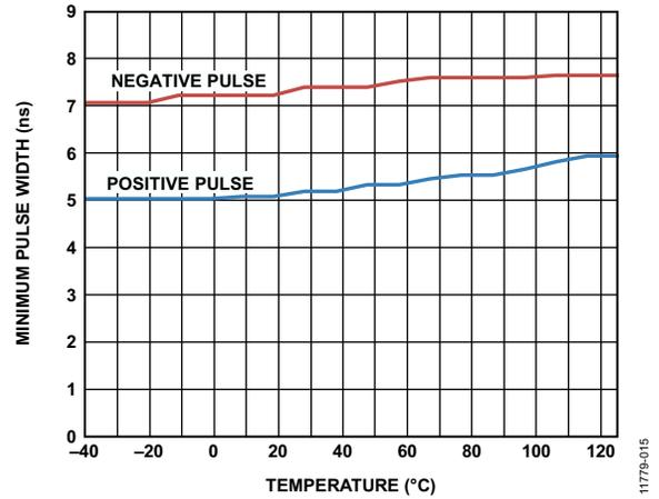
Figure 15. Watchdog Input Minimum Pulse Width vs. Temperature
