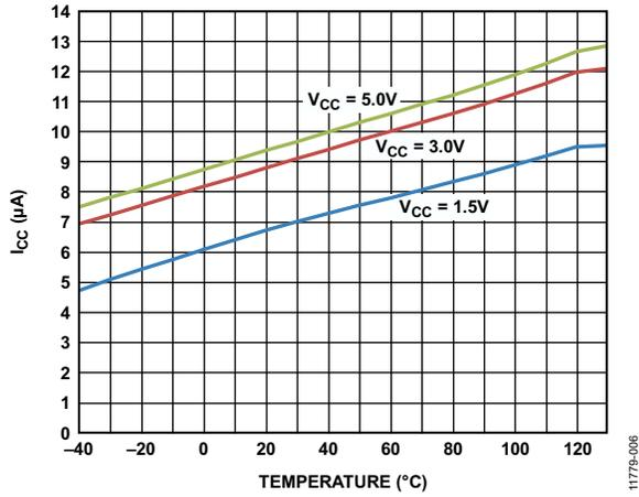
Figure 6. Supply Current ( $I_{CC}$ ) vs. Temperature
