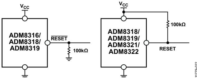
Figure 22. Ensuring Reset Valid to  $V_{CC} = 0$  V
