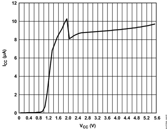
Figure 7. Supply Current ( $I_{CC}$ ) vs. Supply Voltage ( $V_{CC}$ )
