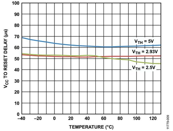
Figure 9.  $V_{CC}$  to Reset Delay vs. Temperature
