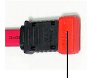
Take out the dust cover and connect to the hard disk devices
