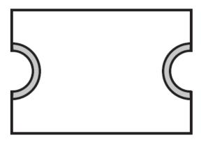
Terminal material: Electroless Ni under immersion Au
