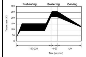
• Recommend reflow methods : IR, vapor phase oven, hot air oven.
