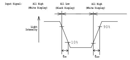
$t_{\rm ON}$ : Turn on time is the time for a photo detector output waveform to go from 90% value to 10% of its maximum.  $t_{\rm OFF}$ : Turn off time is the time for a photo detector output waveform to go from 10% to 90% of its maximum.
