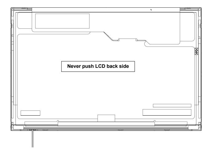
Note) Never push LCD back side. If LCD back side was pressed, It may cause damage of the back light system.
