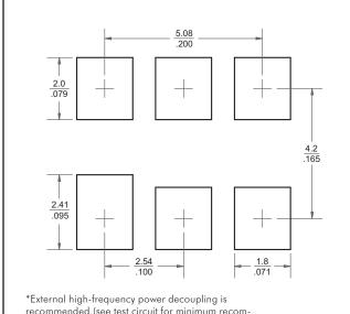
recommended.(see test circuit for minimum recommendation). To ensure optimal performance, do not route traces beneath the package.
