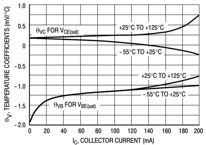
Figure 16. Temperature Coefficients
