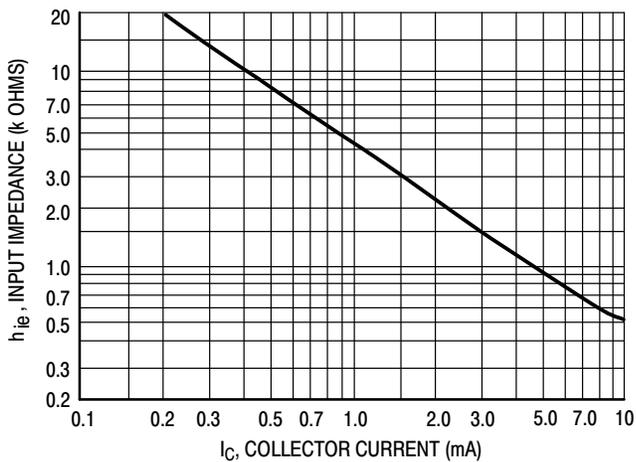
Figure 11. Input Impedance
