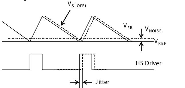
Figure 3—Jitter in PWM Mode
