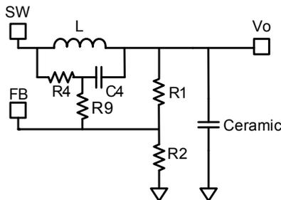
**Figure8—Simplified Circuit of Ceramic Capacitor**
