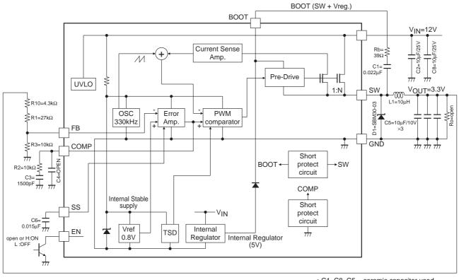
• C1, C8, C5 = ceramic capacitor used. • L1 = CDRH105RPN-100NC (sumida made)
