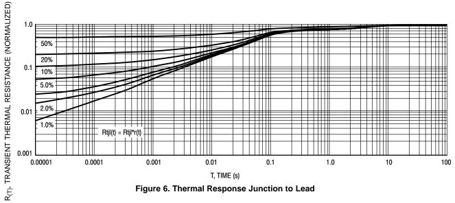
Figure 6. Thermal Response Junction to Lead
