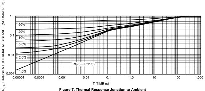
Figure 7. Thermal Response Junction to Ambient
