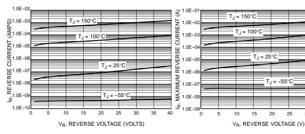
**Figure 3. Typical Reverse Current**
