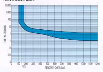
Percent of rated current vs. trip delay at 25° C 200% 1000% % Overload 400% 600% 100% 175% trip in 1 hour Delay Maximum (seconds) no trip 4.5 0.15 0.5 Delay Minimum (seconds) no trip trip in 1 hour
