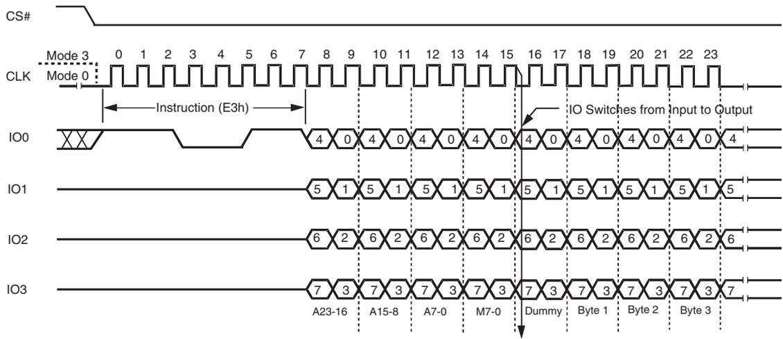
**Figure 7.17** Octal Word Read Quad I/O Instruction Sequence (Previous instruction set M5-4 = 10)
