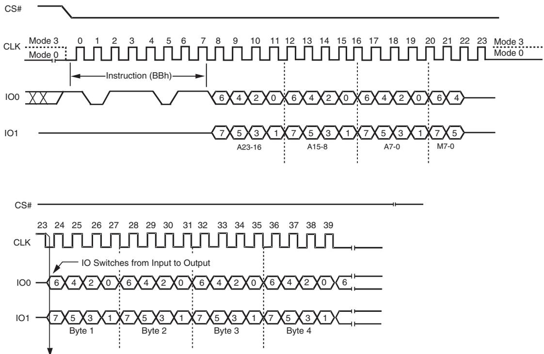
**Figure 7.11** Fast Read Dual I/O Instruction Sequence (Previous instruction set M5-4 = 10)
