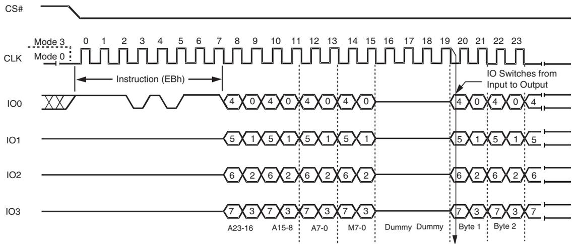
**Figure 7.13** Fast Read Quad I/O Instruction Sequence (Previous instruction set M5-4 = 10)
