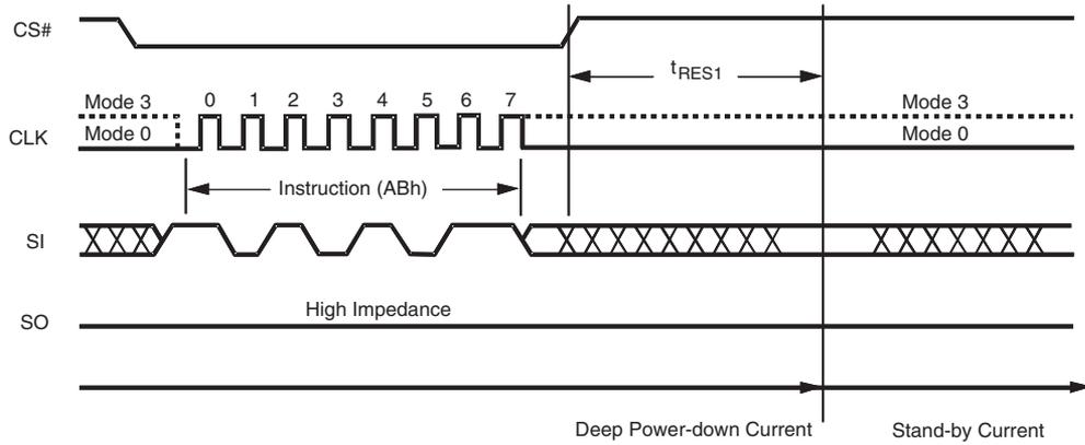
**Figure 7.30** Release from Deep Power-down / Device ID Instruction Sequence Diagram
