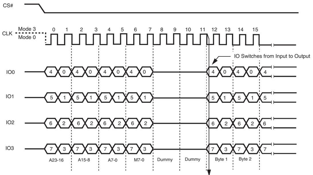
**Fast Read Quad I/O with “8/16/32/64-Byte Wrap Around”**
