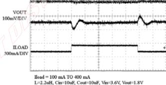
Load Transient Response Idle Mode to PWM Mode
