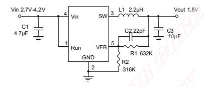
Fig.1 Basic Application Circuit with LSP3100 adjustable version
