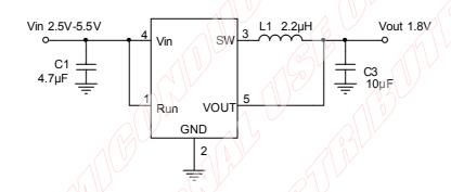
Fig.2 Basic Application Circuit with fixed output versions
