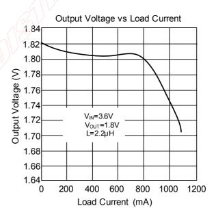
1.5MHZ, 800mA Synchronous Step-Down Converter
