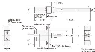
\* Vinyl-insulated round cable of 3.5 dia., 3 cores, (0.14 mm² with 1.0-dia. insulator); Standard length: 1 m
