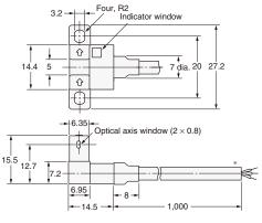
\* Vinyl-insulated round cable of 3.5 dia., 3 cores, (0.14 mm² with 1.0-dia. insulator); Standard length: 1 m
