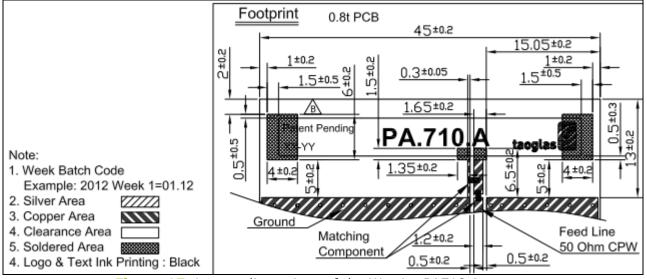
Figure 15. Layout dimensions of the Warrior PA710 Antenna.
