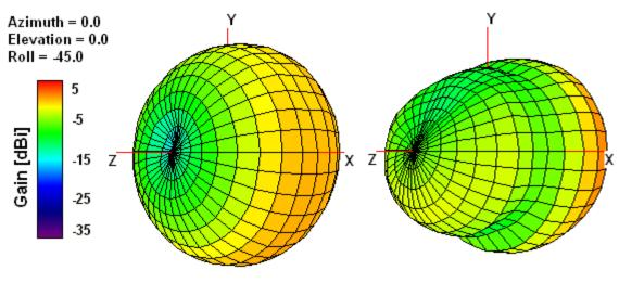
1805 MHz1910 MHzFigure 9. 3D Radiation Pattern at 1805 and 1910 MHz of the Warrior PA710 Antenna
