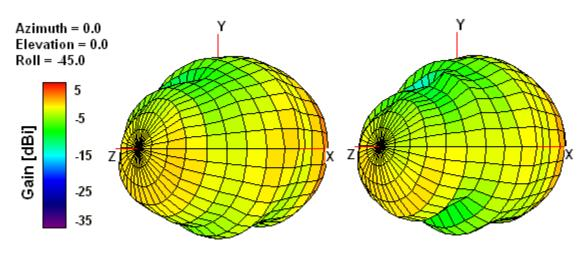
2600 MHz2700 MHzFigure 12. 3D Radiation Pattern at 2700 and 2800 MHz of the Warrior PA710 Antenna
