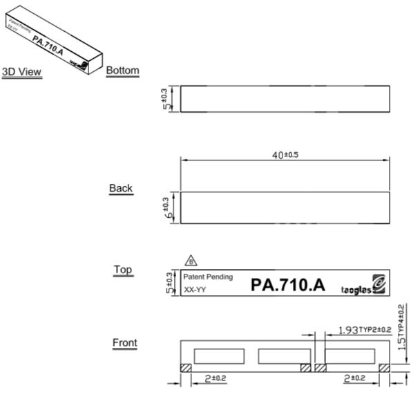
Figure 14. Mechanical Drawing of the Warrior PA710 Antenna.
