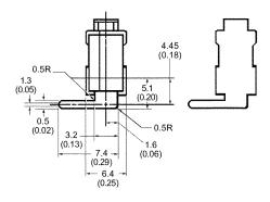
Note: Thickness of all the terminals is 0.5 mm.
