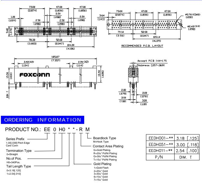
EE Series Vertical Type W/O Retainer, Metal H/D 1.00mm [.039"] Pitch 340 Pos.
