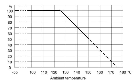
The above diagram is only valid for MLV with conductive adhesive technology.
