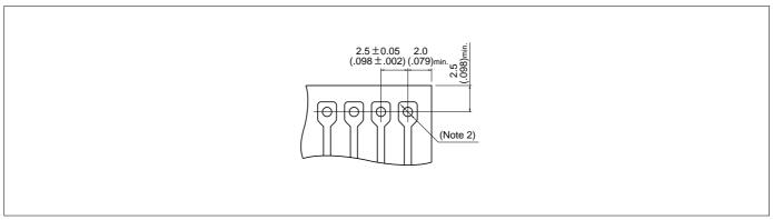
1. Applicable PC board thickness: Type A 1.6mm(.063")
