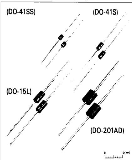
$V_{FM}\leq 1.1\sim 1.5V$ ,  $t_{rr}\leq 200ns$ . Optimum for secondary rectification of switching power supplies for TVs and monitors or secondary rectification of flyback transformers.
