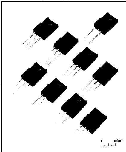
The height of these HEDs is approximately 2 mm less than that of conventional packages, and there is no conductive exposure on the mold surface. They are built into the TO-220(N)IS, the new insulating package version of the TO-220.
