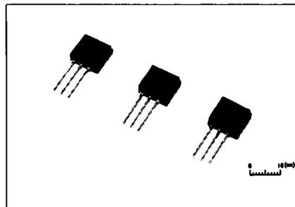
High-speed rectifier in a TO-220FL package with a maximum height of only 13.1 mm. These devices are used in ultrathin system units such as 1-inch power supplies.
