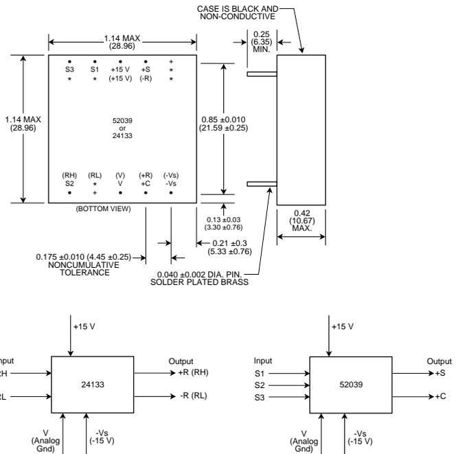
The mechanical outline is the same for the synchro input transformer (52039) and the reference input transformer (24133), except for the pins. Pins for the reference transformer are shown in parenthesis ( ). An asterisk \* indicates that the pin is omitted.
