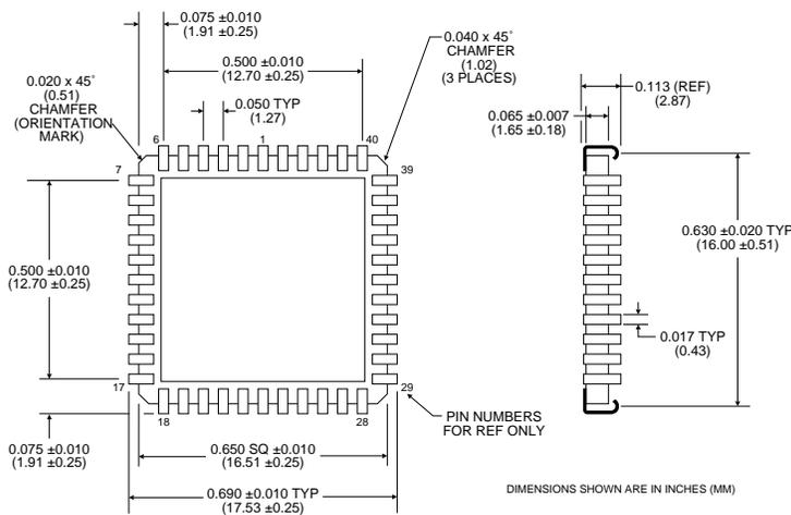
**FIGURE 18. RDC-19222S (44-PIN CERAMIC J-LEAD) MECHANICAL OUTLINE**
