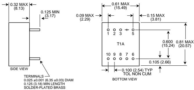
**FIGURE 6C. TRANSFORMER LAYOUT AND SCHEMATIC (REFERENCE INPUT - B-426)**
