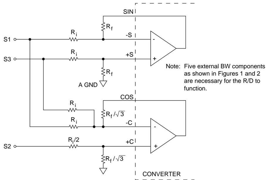
$$\frac{R_i}{R_f} \times 2 V_{rms} = \text{Resolver L-L rms voltage}$$
