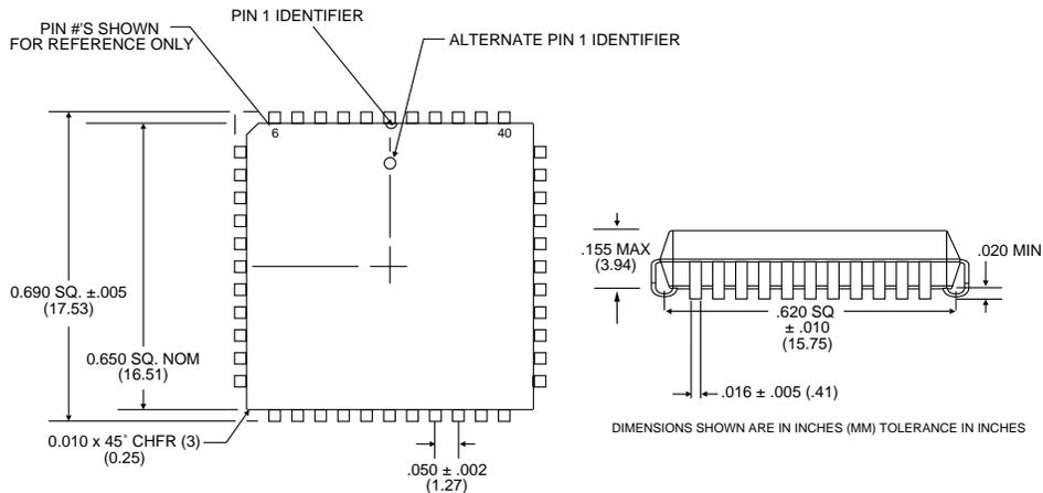
**FIGURE 17. RDC-19222S (44-PIN PLASTIC J-LEAD) MECHANICAL OUTLINE**
