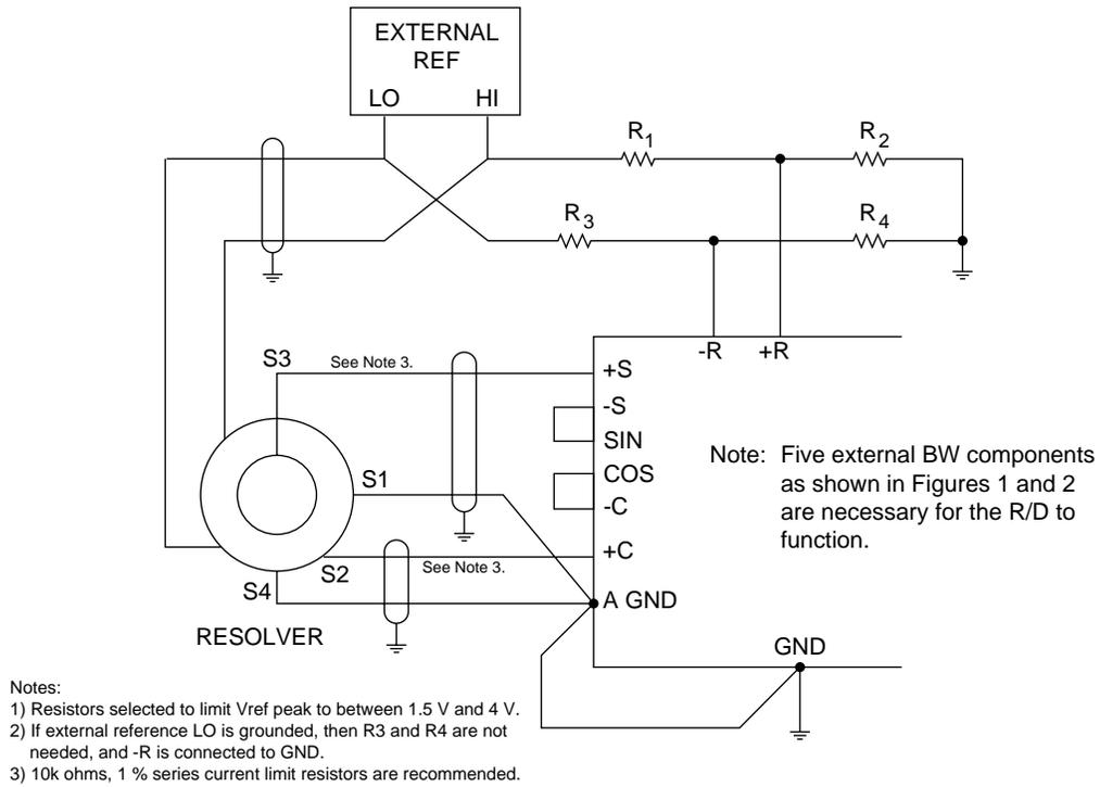
**FIGURE 8. TYPICAL CONNECTIONS, 2 VOLT RESOLVER, DIRECT INPUT**
