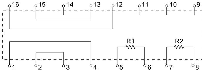
**FIGURE 19. (DDC-55688-1) LAYOUT AND RESISTOR VALUES (R1 AND R2 = 10 KΩ 1.0% TOL, ABSOLUTE TC = ±100 PPM MAX)**
