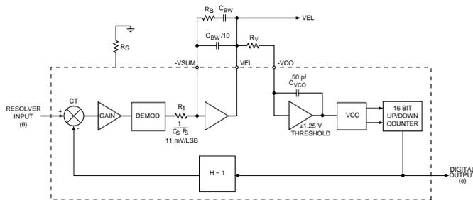
FIGURE 2. TRANSFER FUNCTION BLOCK DIAGRAM #1
