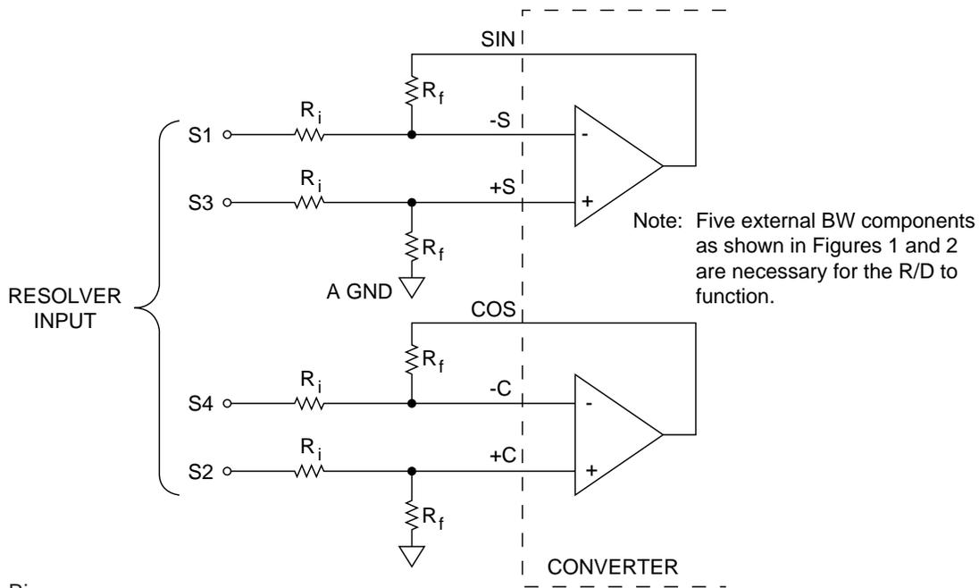
$$\frac{R_i}{R_f} \times 2 V_{rms} = \text{Resolver L-L rms voltage}$$
