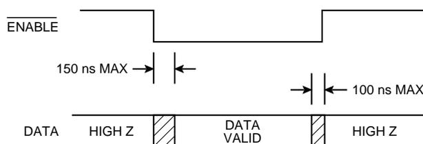
FIGURE 14. ENABLE TIMING
