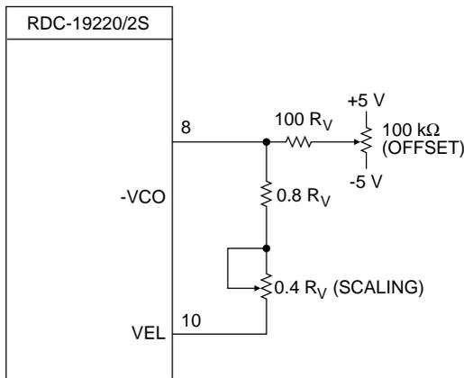
FIGURE 11. VELOCITY TRIMMING
