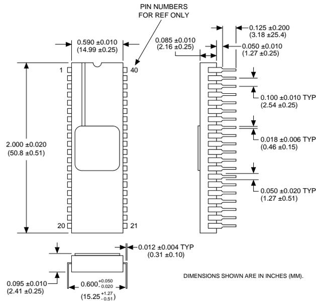
**FIGURE 16. RDC-19220S (40-PIN DDIP) CERAMIC PACKAGE MECHANICAL OUTLINE**
