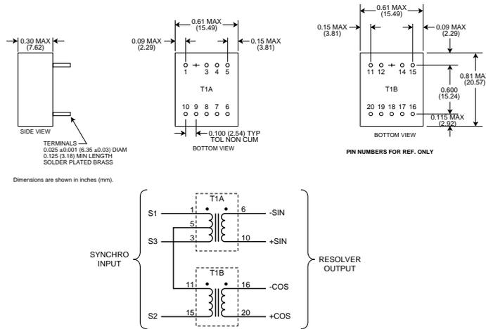
**FIGURE 6A. TRANSFORMER LAYOUT AND SCHEMATIC (SYNCHRO INPUT - 52034/52035)**
