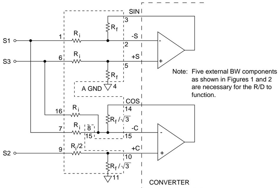
S1, S2, and S3 should be triple twisted shielded; RH and RL should be twisted shielded. In both cases the shield should be tied to AGND at the converter.
