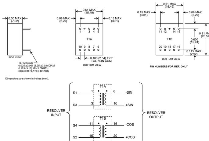
**FIGURE 6B. TRANSFORMER LAYOUT AND SCHEMATIC (RESOLVER INPUT - 52036/52037/52038)**
