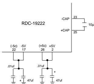
**FIGURE 5. -5V BUILT-IN INVERTER**
