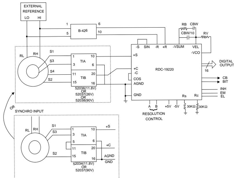
**FIGURE 7. TYPICAL TRANSFORMER CONNECTIONS**
