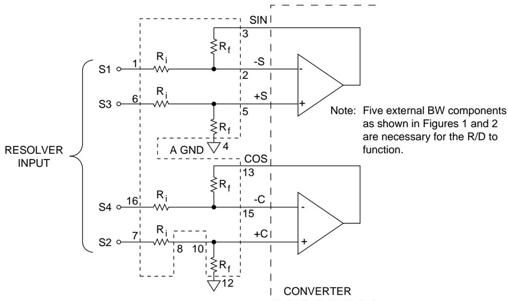
S1 and S3, S2 and S4, and RH and RL should be ideally twisted shielded, with the shield tied to AGND at the converter.
