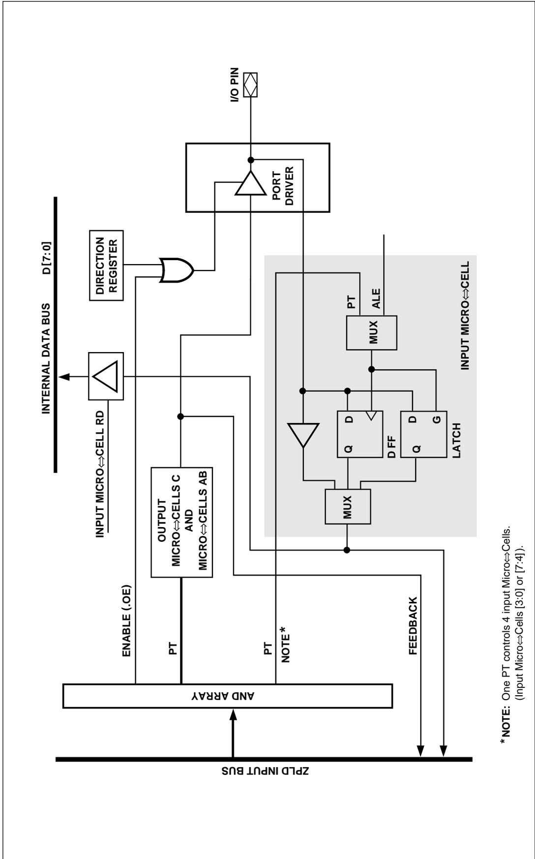
\* NOTE: One PT controls 4 input Micro↔Cells.
