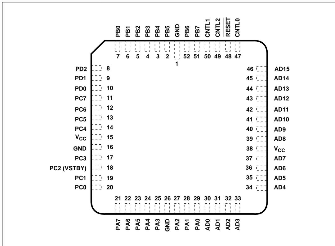
**Figure 47 Drawing L6 – 52-Pin Ceramic Leaded Chip Carrier (CLDCC)
