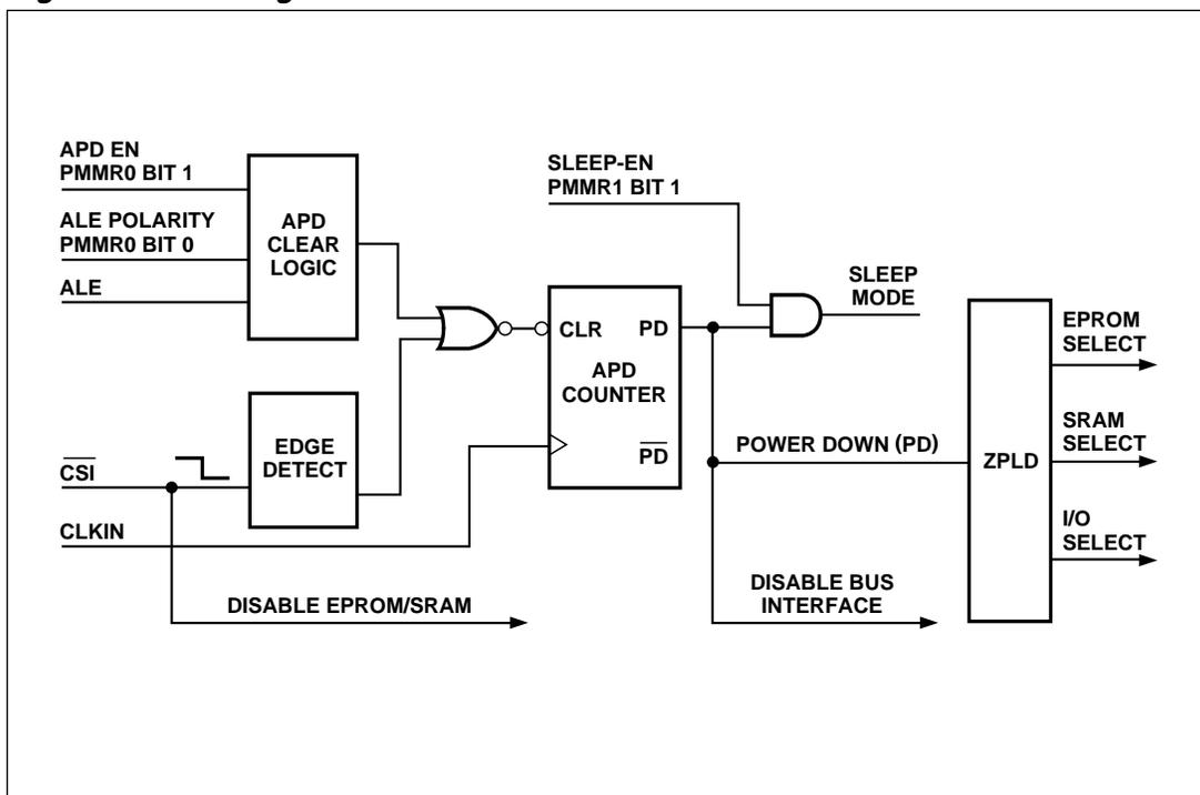
**Figure 29. Enable Power Down Flow Chart**
