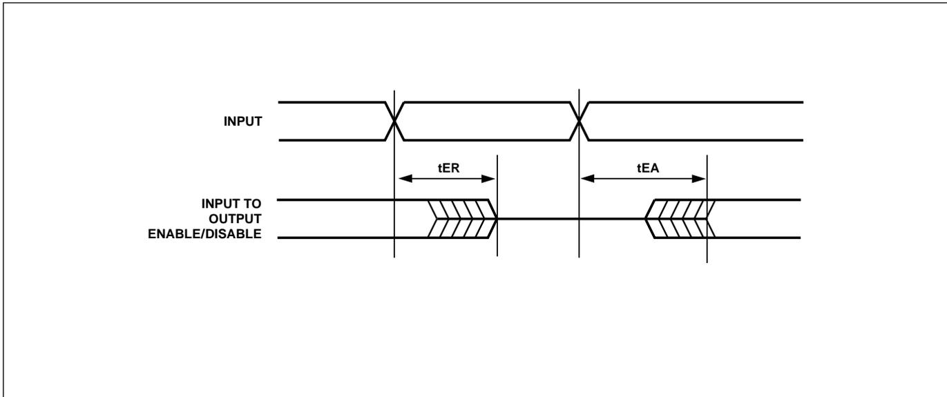
Figure 41. Asynchronous Reset/Preset
