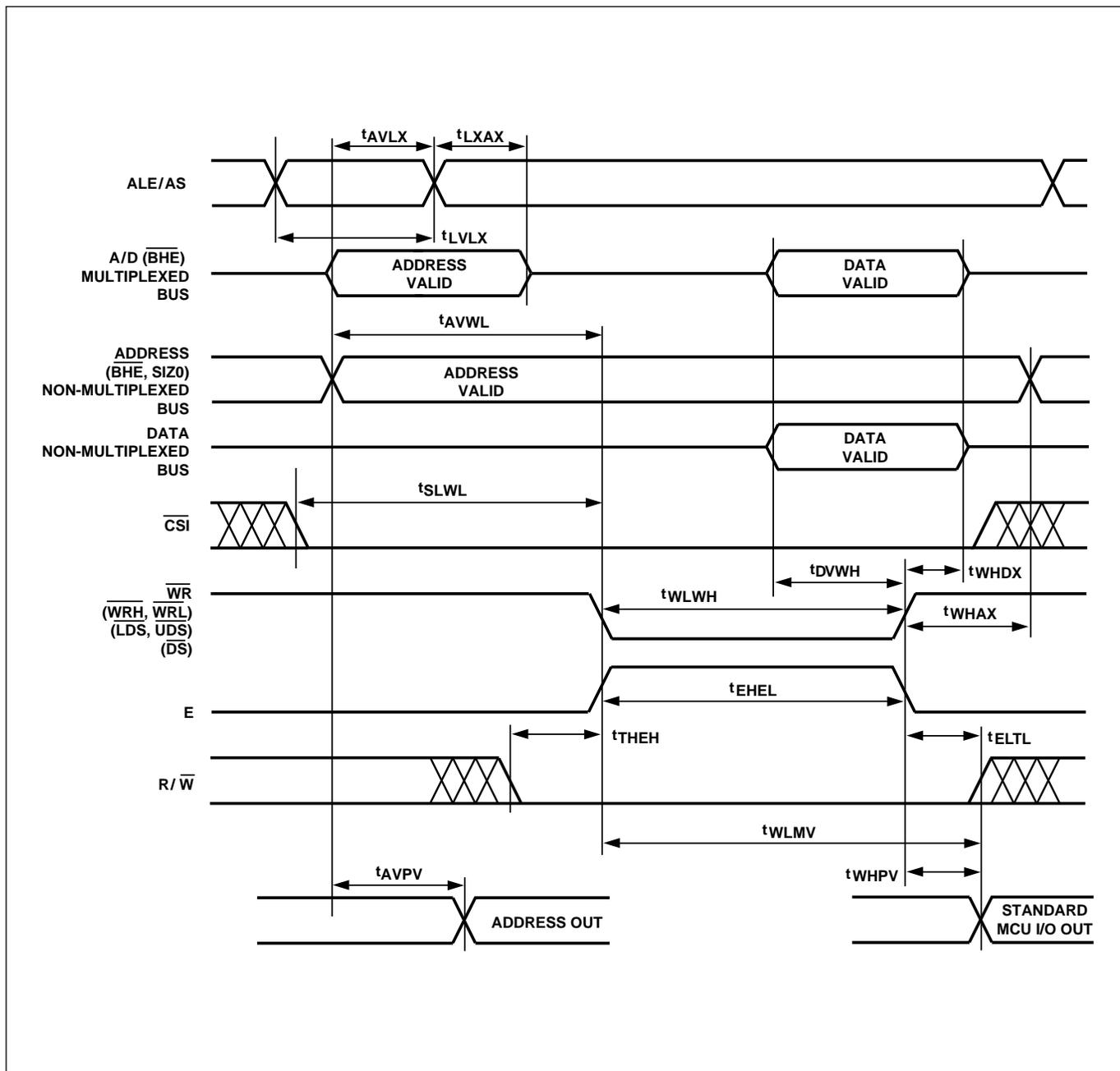
**Figure 34. Peripheral I/O Read Timing**
