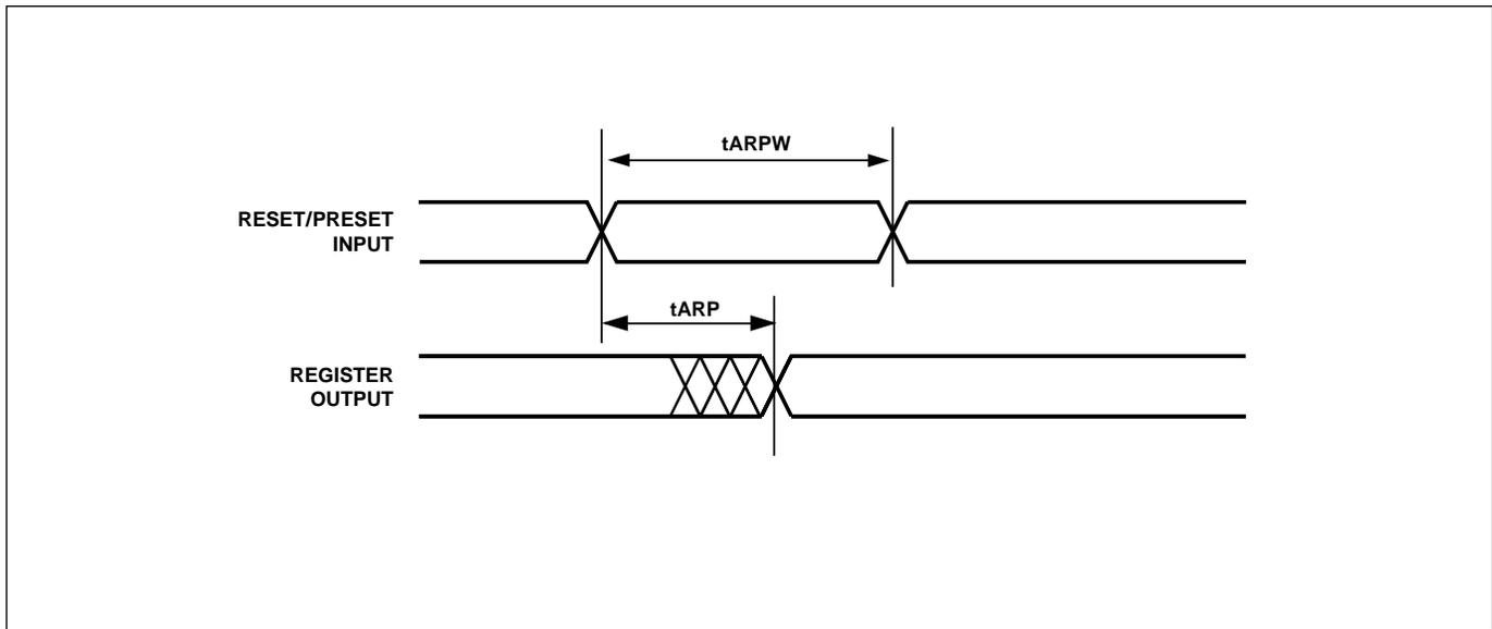
**Figure 42. Reset Timing**
