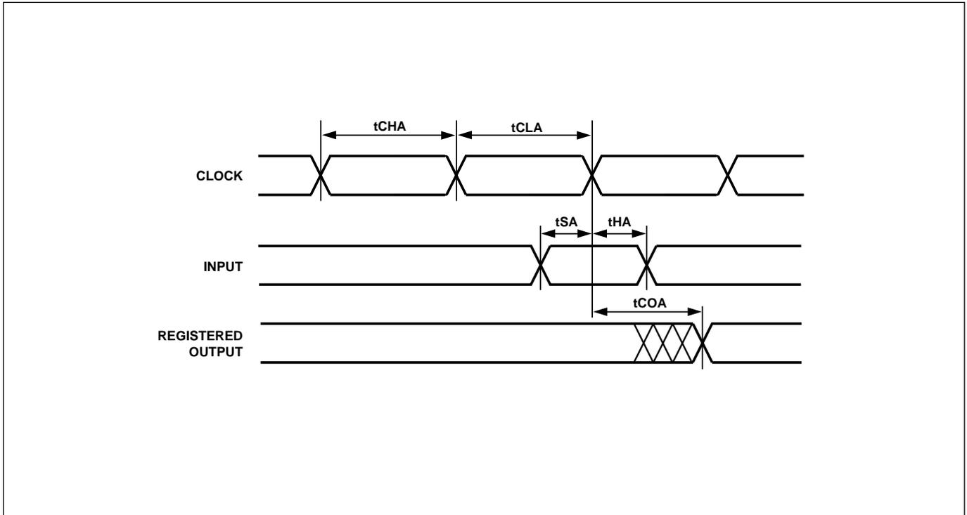
**Figure 39. Input Micro↔Cell Timing (Product-Term Clock)**
