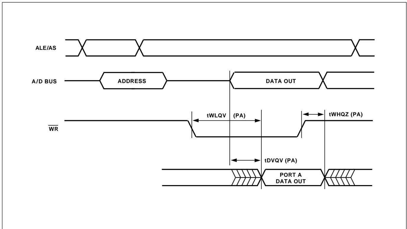
**Figure 36. Combinatorial Timing – ZPLD**
