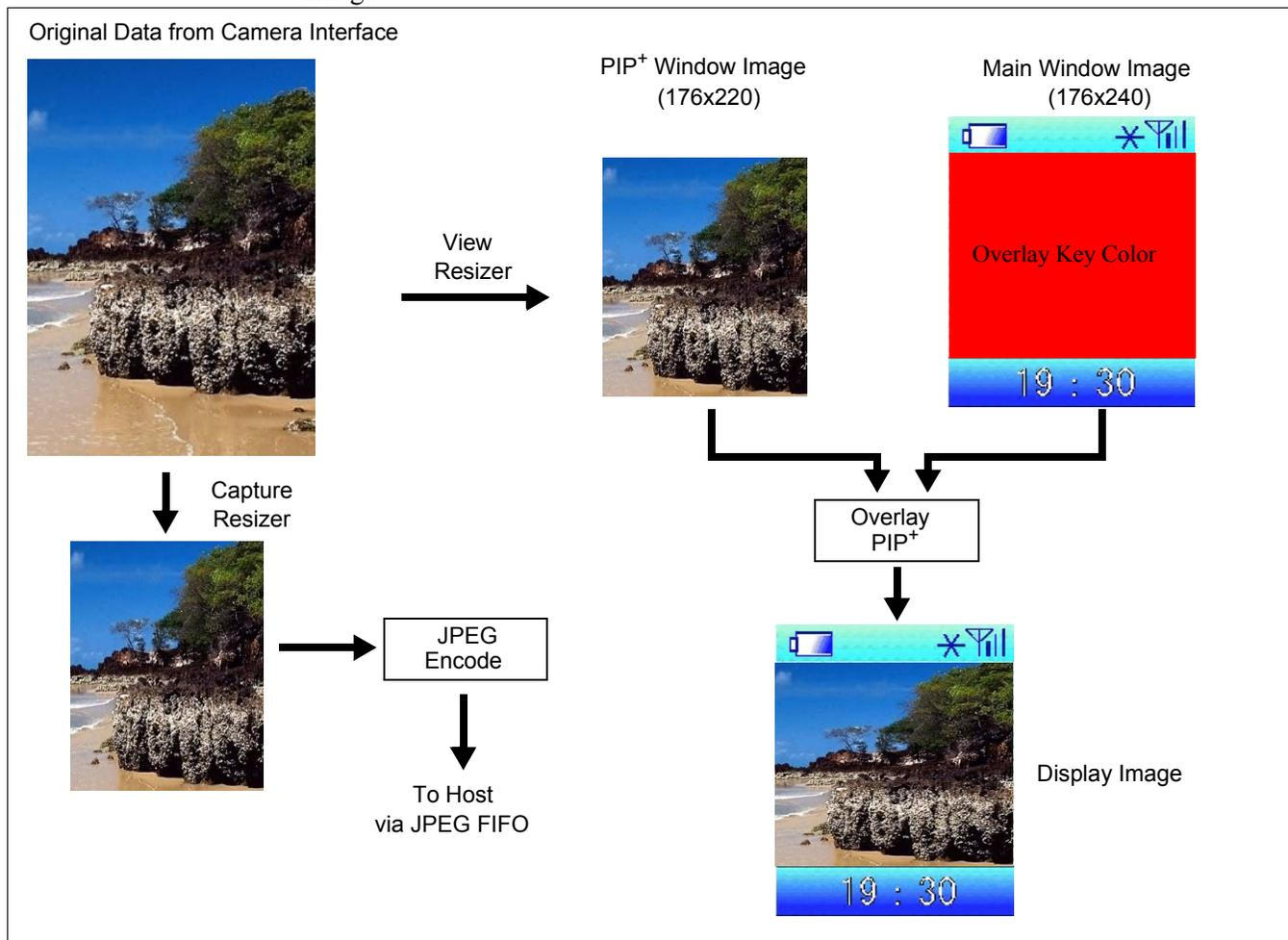
Figure 8-9: Main Window, PIP<sup>+</sup> Window, Overlay, and JPEG
