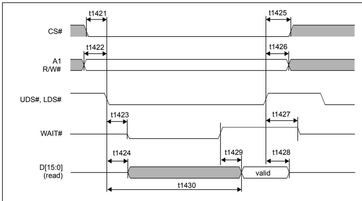
Figure 7-28: Indirect 68 Interface Read Cycle Timing (Wait Mode)
