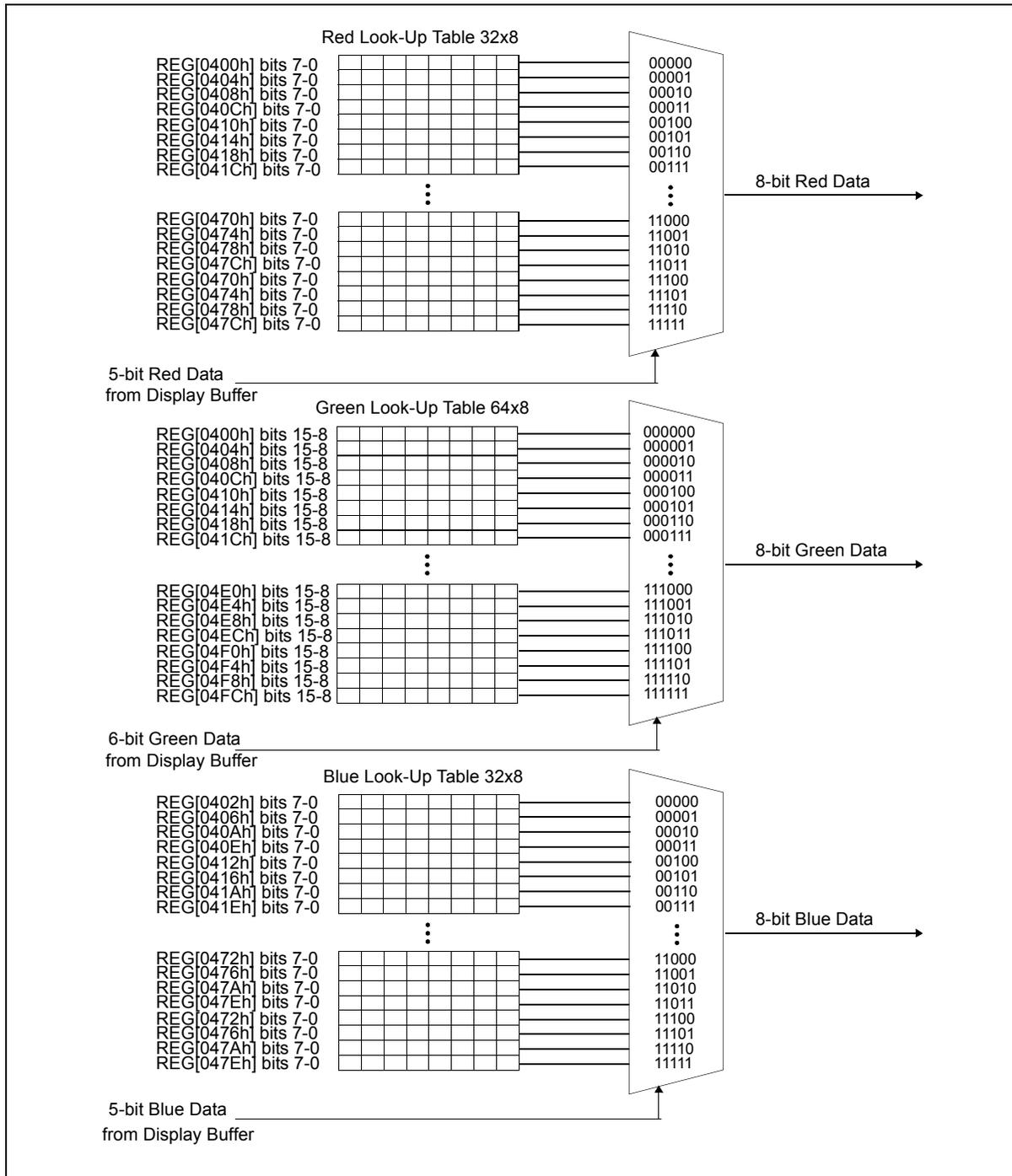
Figure 12-3: LUT1 (Main Window) for 16 Bpp Architecture
