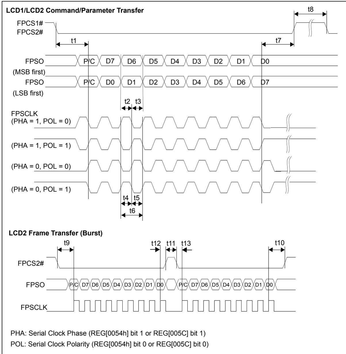
Figure 7-34: LCD1 ND-TFD, LCD2 9-Bit Serial Interface Timing
