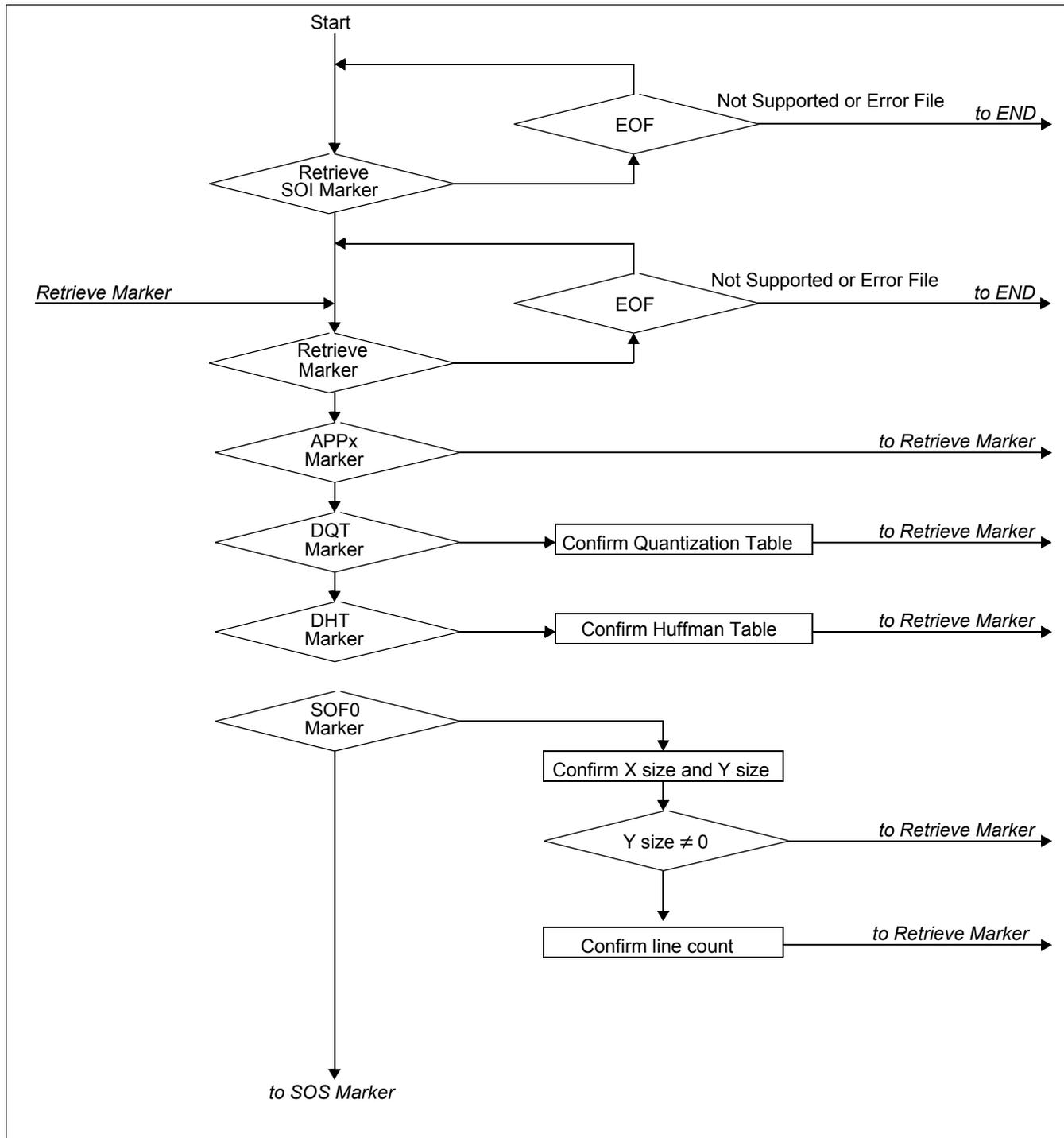
Figure 19-6: JPEG Decoding Process (1 of 6)
