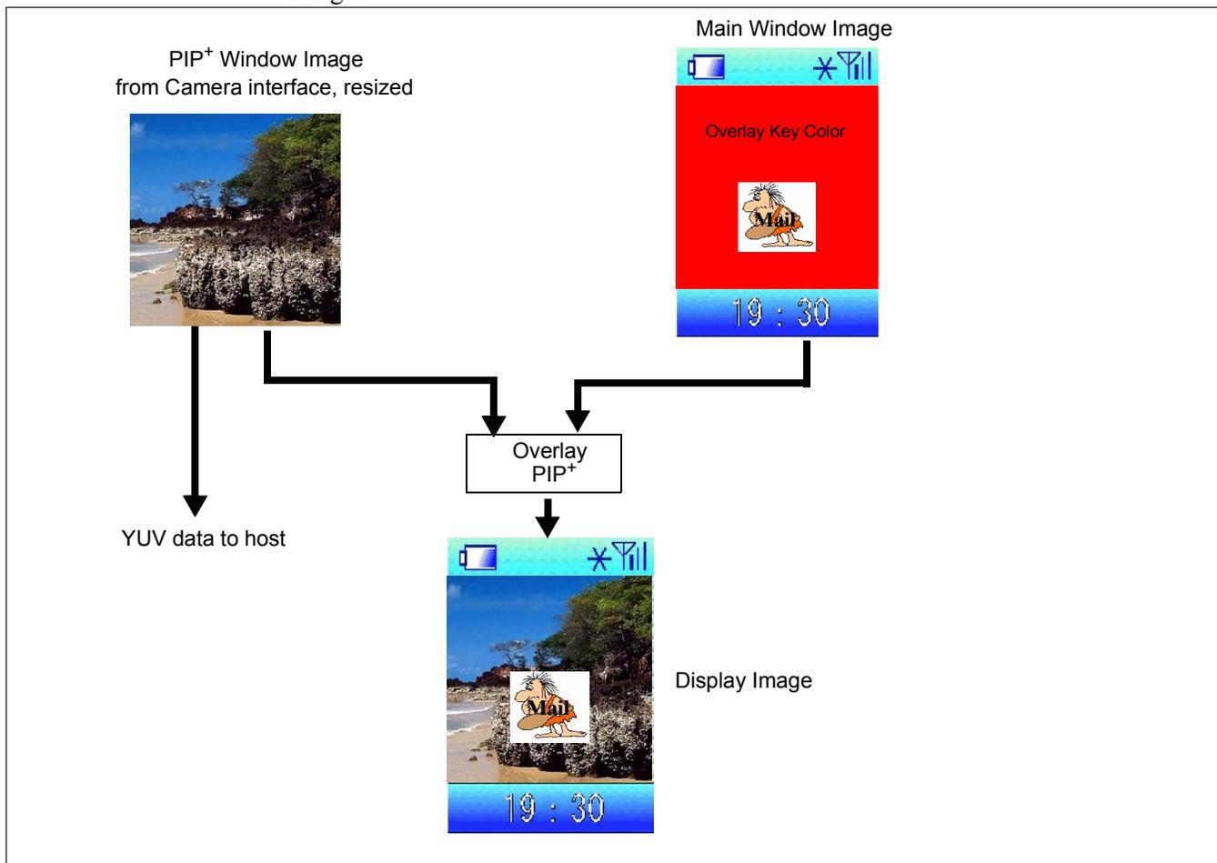
Figure 8-7: Main Window, PIP<sup>+</sup> Window, Overlay, and YUV
