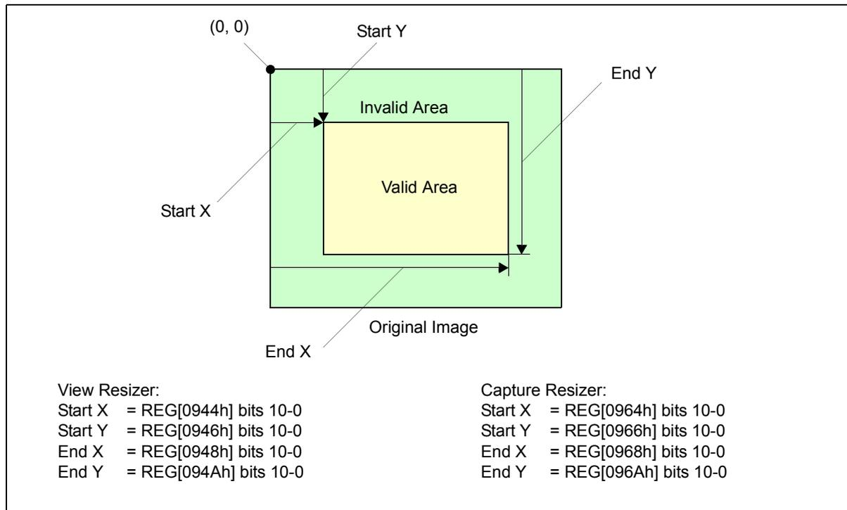
*Figure 17-1: Trimming Function*
