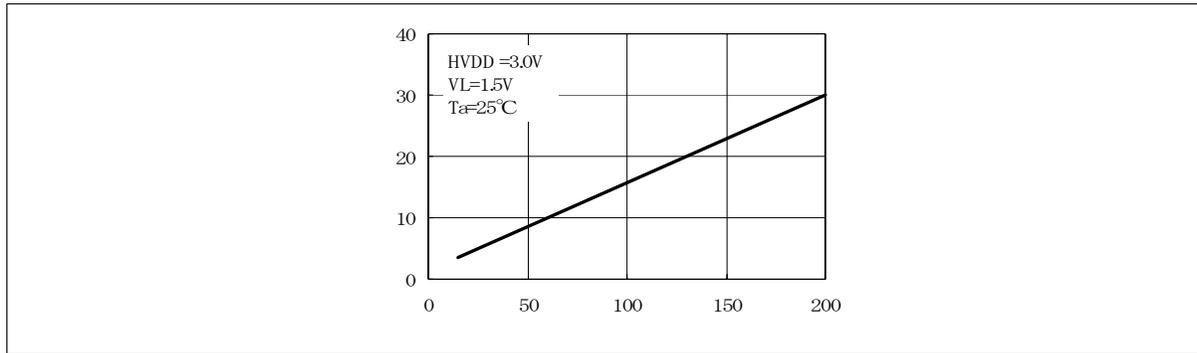
Figure 7-39: Rise Time v.s. Capacitance ( $C_L$ )
