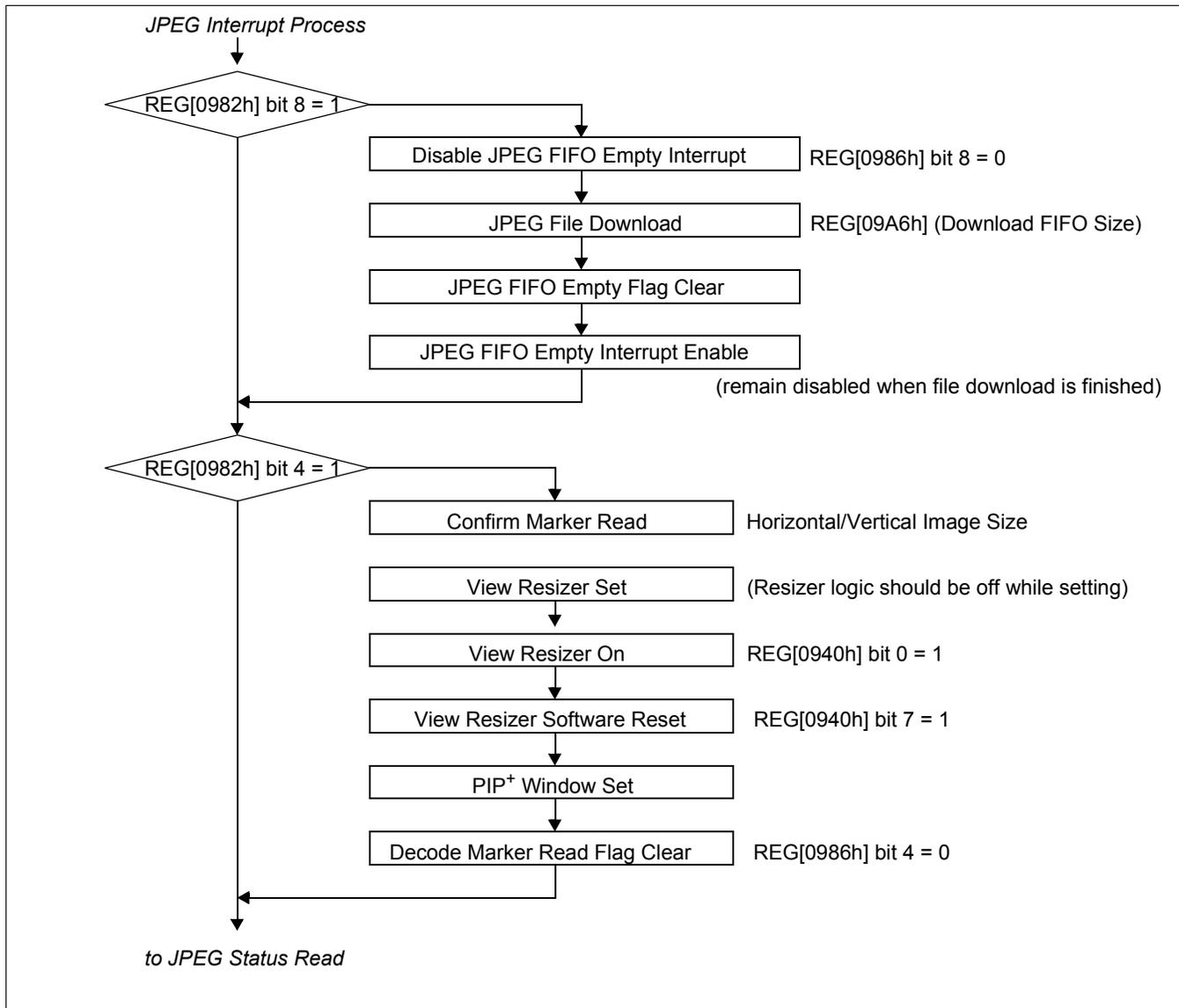
*Figure 19-10: JPEG Decoding Process (5 of 6)*
