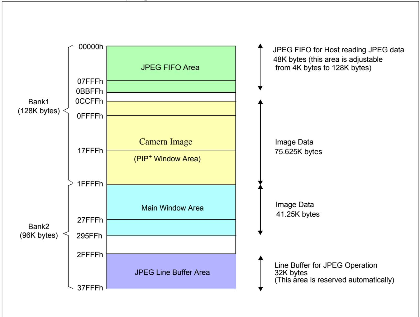
Figure 8-10: Memory Map for Main Window, PIP+ Window, Overlay and JPEG
