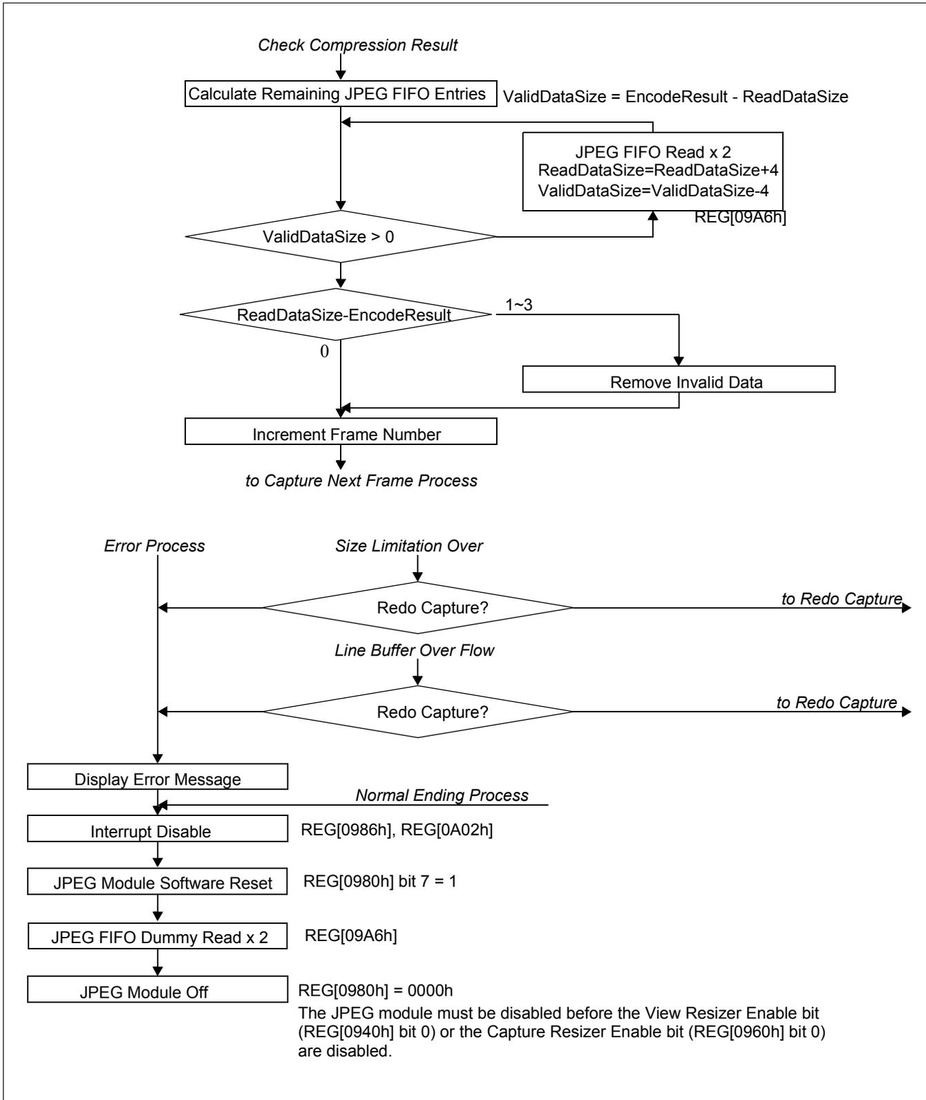
Figure 19-5: JPEG Encoding Process (4 of 4)
