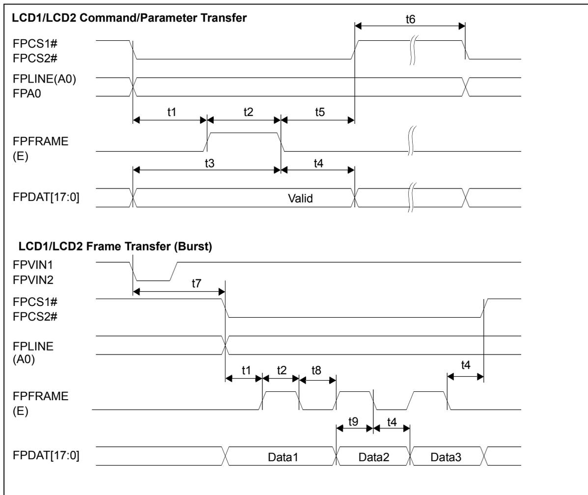
Figure 7-38: LCD1, LCD2 Parallel Interface Timing (68)
