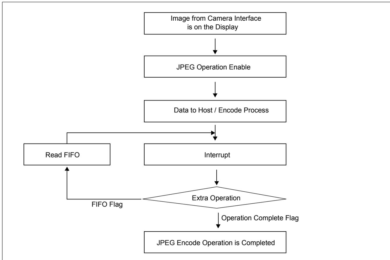
Figure 18-3: JPEG Encode Data from the Camera Interface
