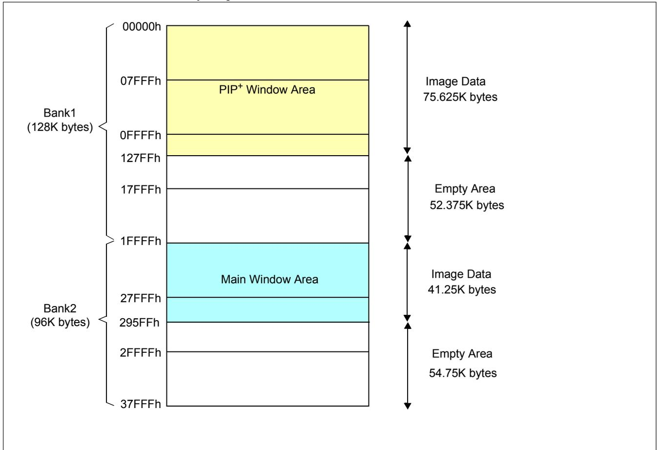
Figure 8-6: Memory Map for Main Window, PIP+ Window, and Overlay Display
