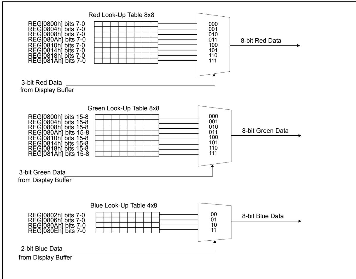
Figure 12-2: LUT2 (PIP<sup>+</sup> Window) for 8 Bpp Architecture
