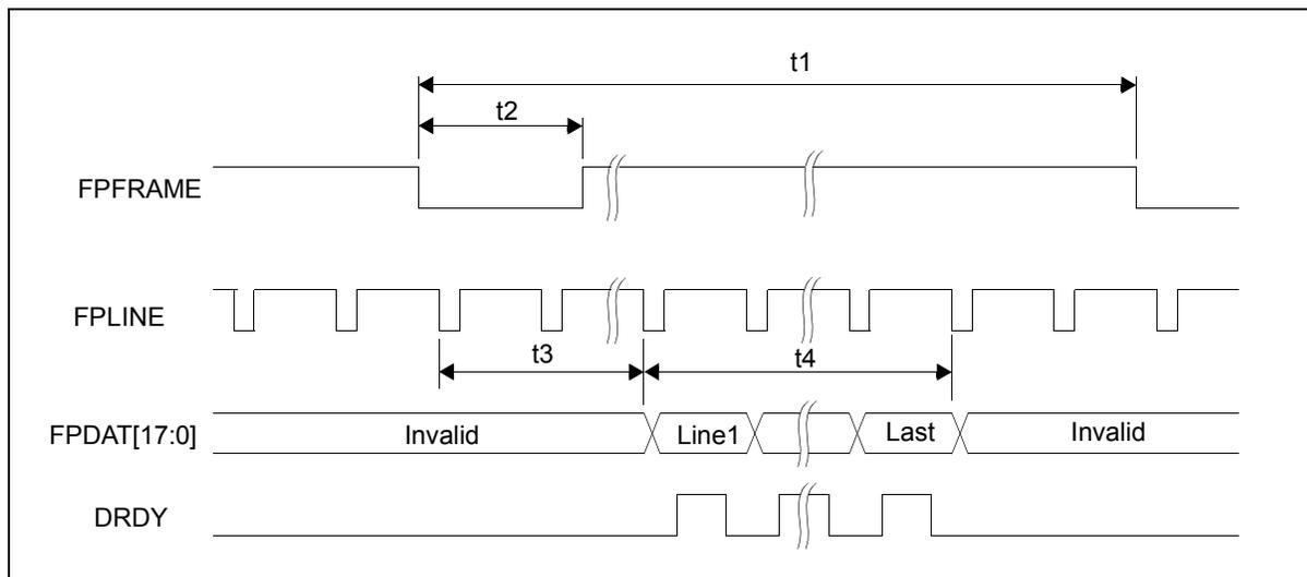
Figure 7-32: Generic RGB Type Interface Panel Vertical timing
