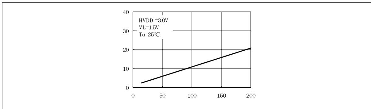
Figure 7-40: Fall Time V.s. Capacitance ( $C_L$ )
