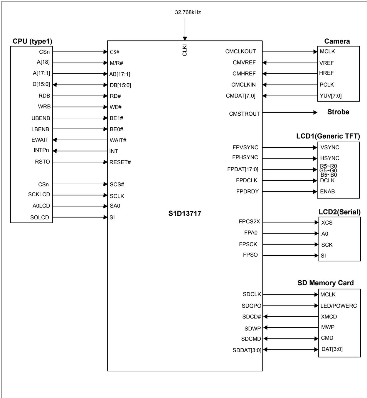
Figure 3-1: SID13717 System Diagram 1
