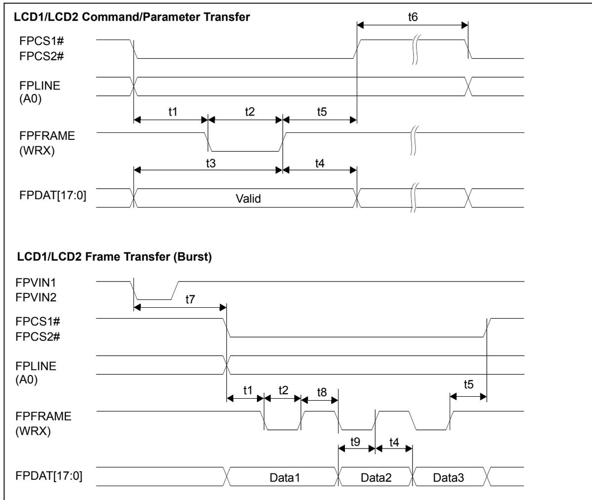
Figure 7-37: LCD1, LCD2 Parallel Interface Timing (80)
