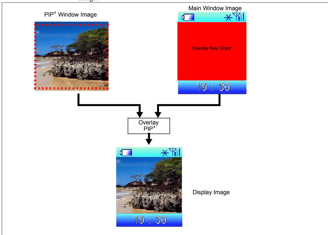
Figure 8-5: Main Window, PIP<sup>+</sup> Window, and Overlay Display
