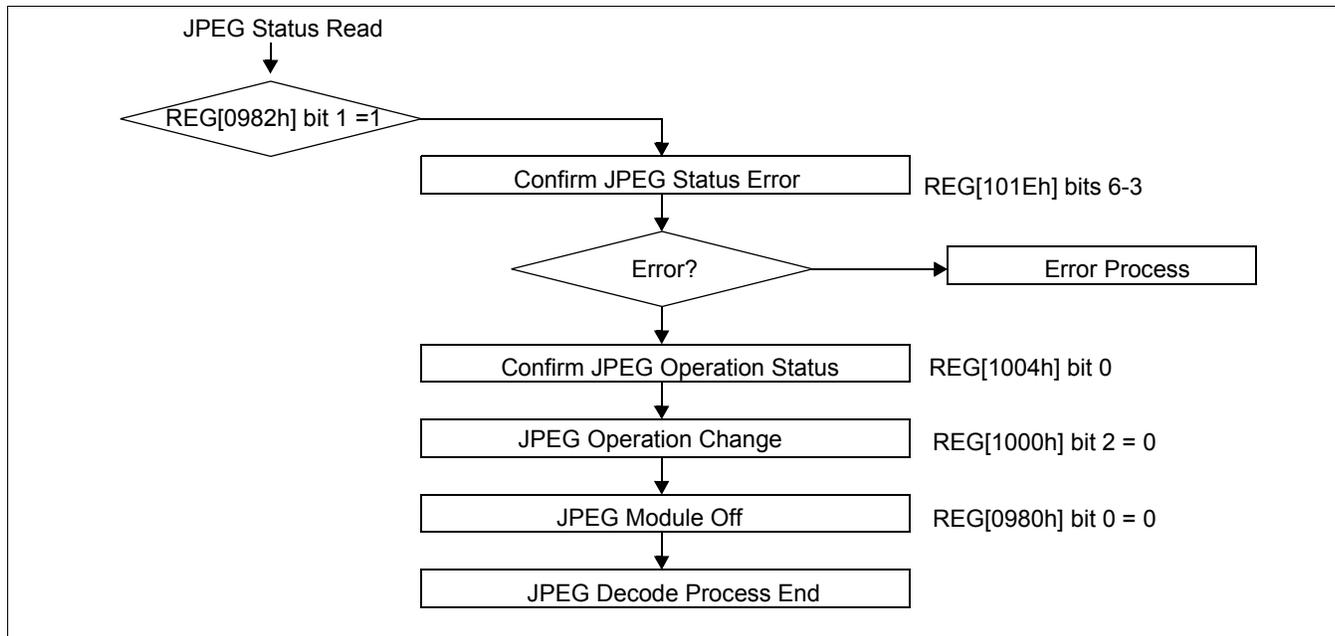
Figure 19-11: JPEG Decoding Process (6 of 6)
