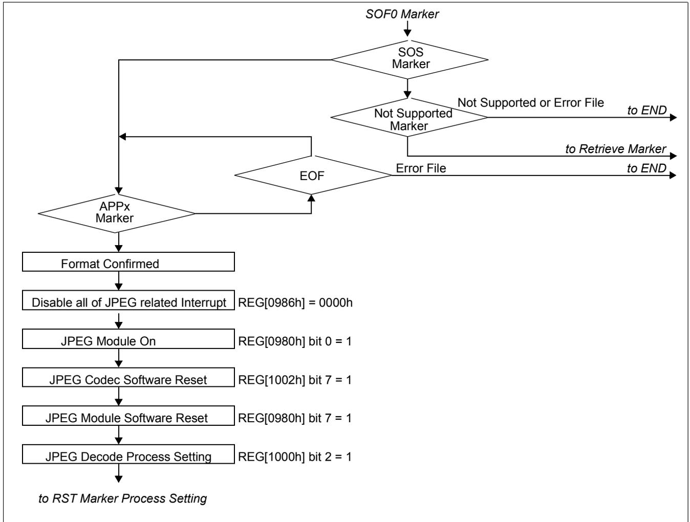
Figure 19-7: JPEG Decoding Process (2 of 6)
