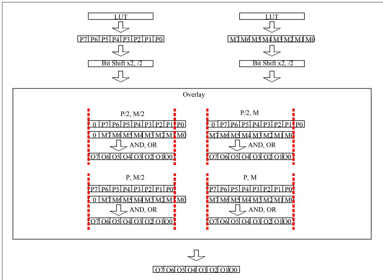
Figure 15-5: Data Flow for Bit Shift Function
