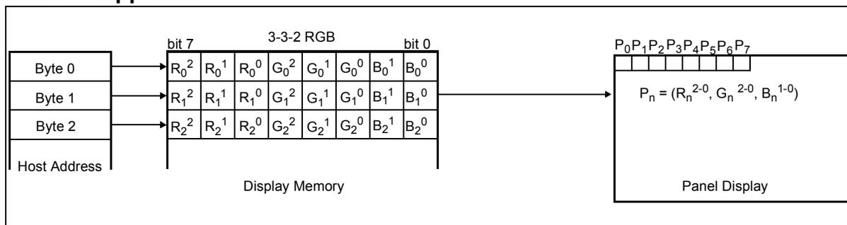
Figure 13-5: LUT Bypass for 8 Bpp mode
