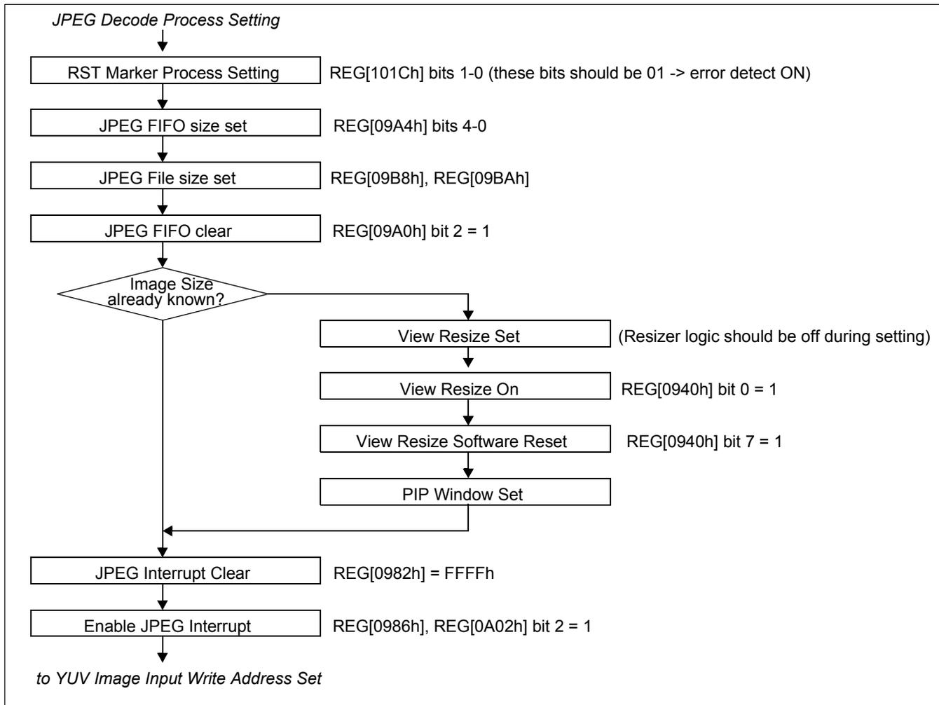
Figure 19-8: JPEG Decoding Process (3 of 6)
