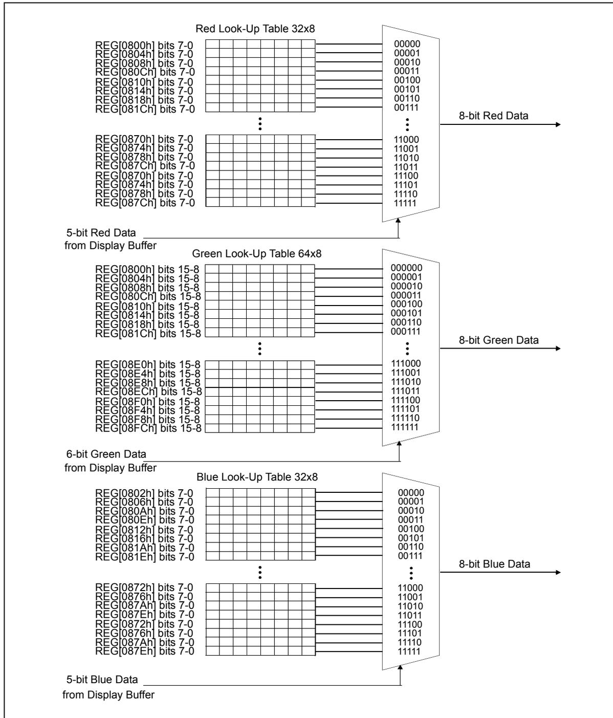
Figure 12-4: LUT2 (PIP<sup>+</sup> Window) for 16 Bpp Architecture
