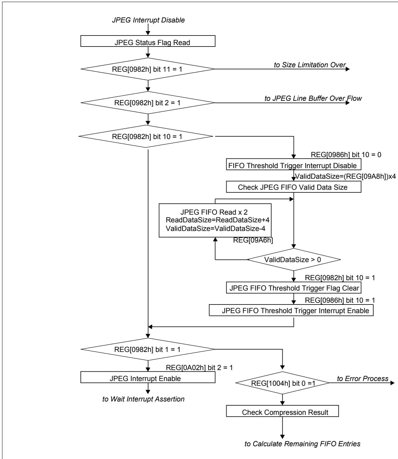
Figure 19-4: JPEG Encoding Process (3 of 4)
