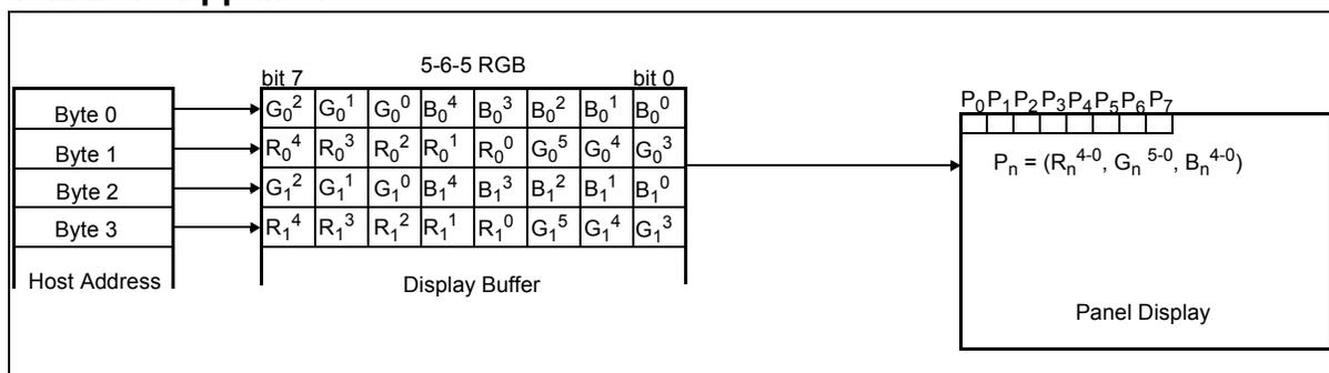
Figure 13-6: LUT Bypass for 16 Bpp mode
