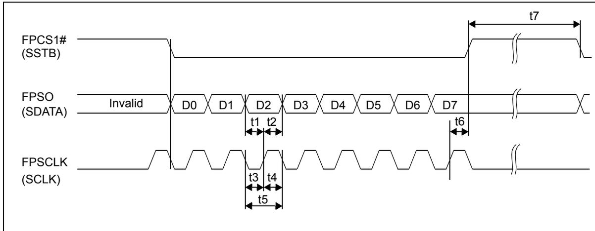
Figure 7-35: LCD1 a-Si TFT Serial Interface Timing
