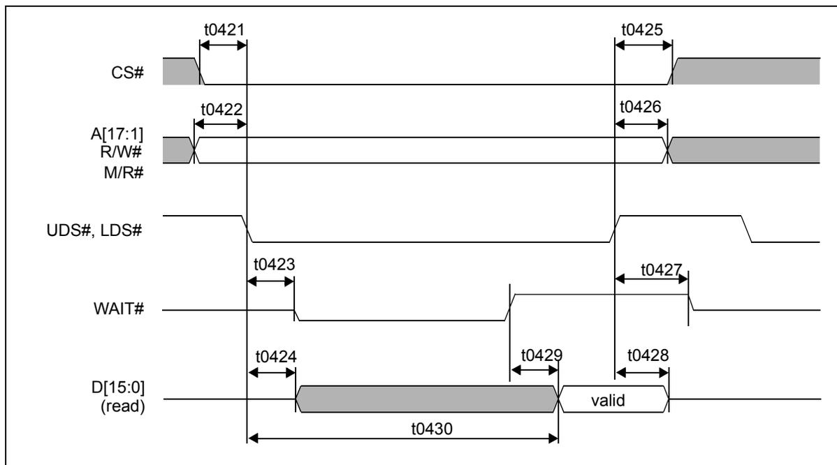
Figure 7-16: Direct 68 Interface Read Cycle Timing (Wait Mode)
