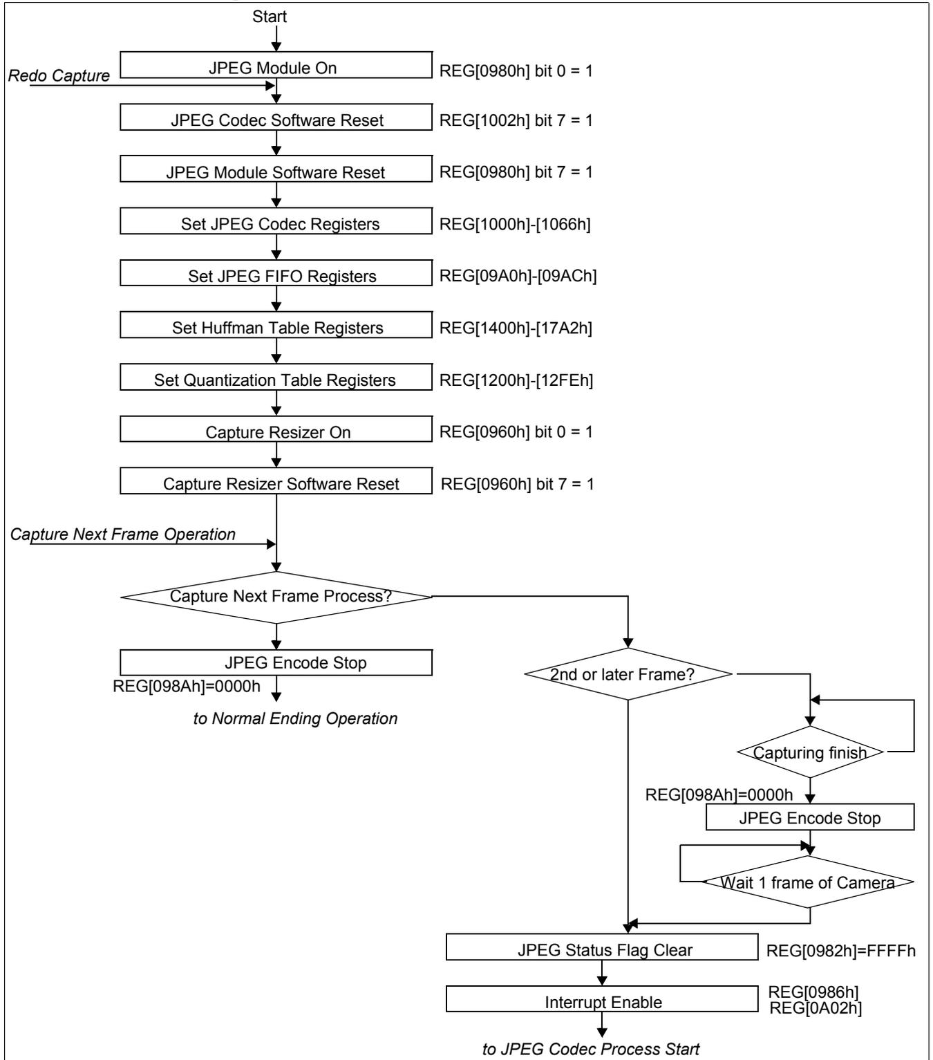
Figure 19-2: JPEG Encoding Process (1 of 4)
