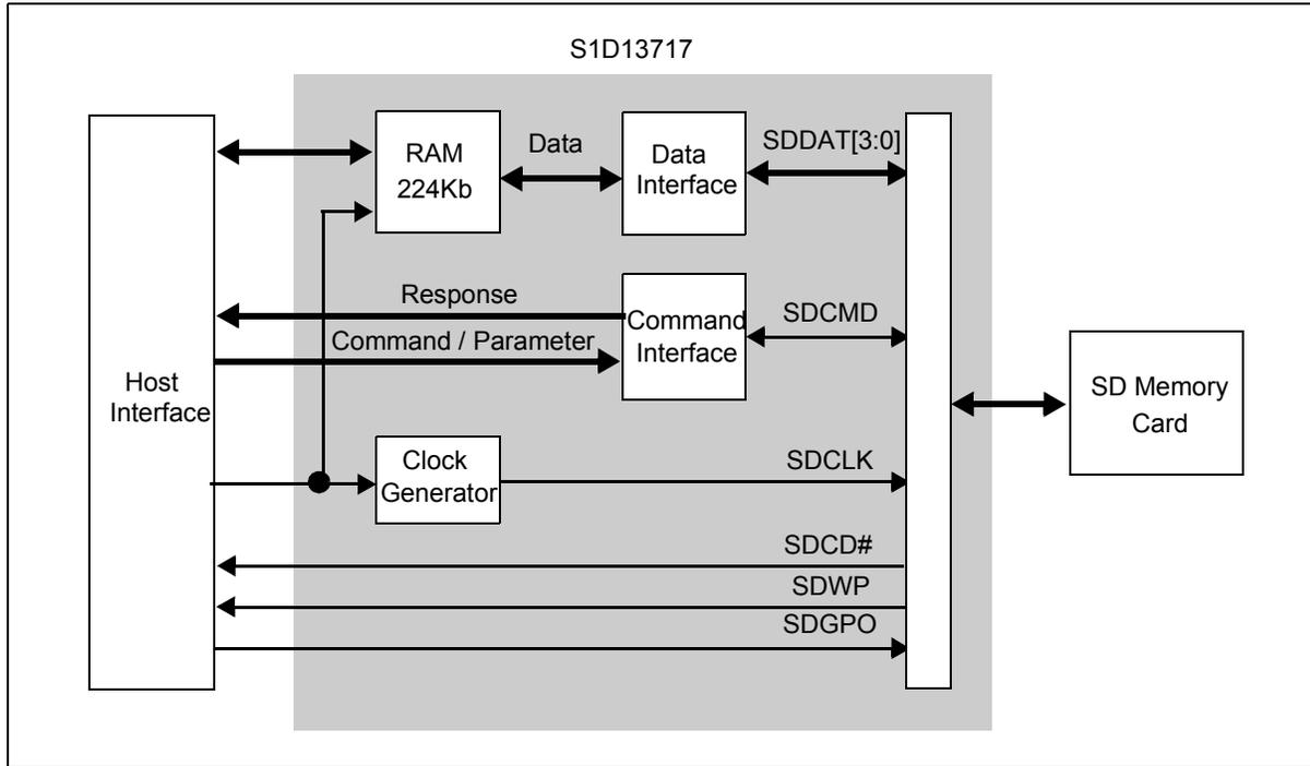
Figure 21-1: SD Memory Card Interface Block Diagram
