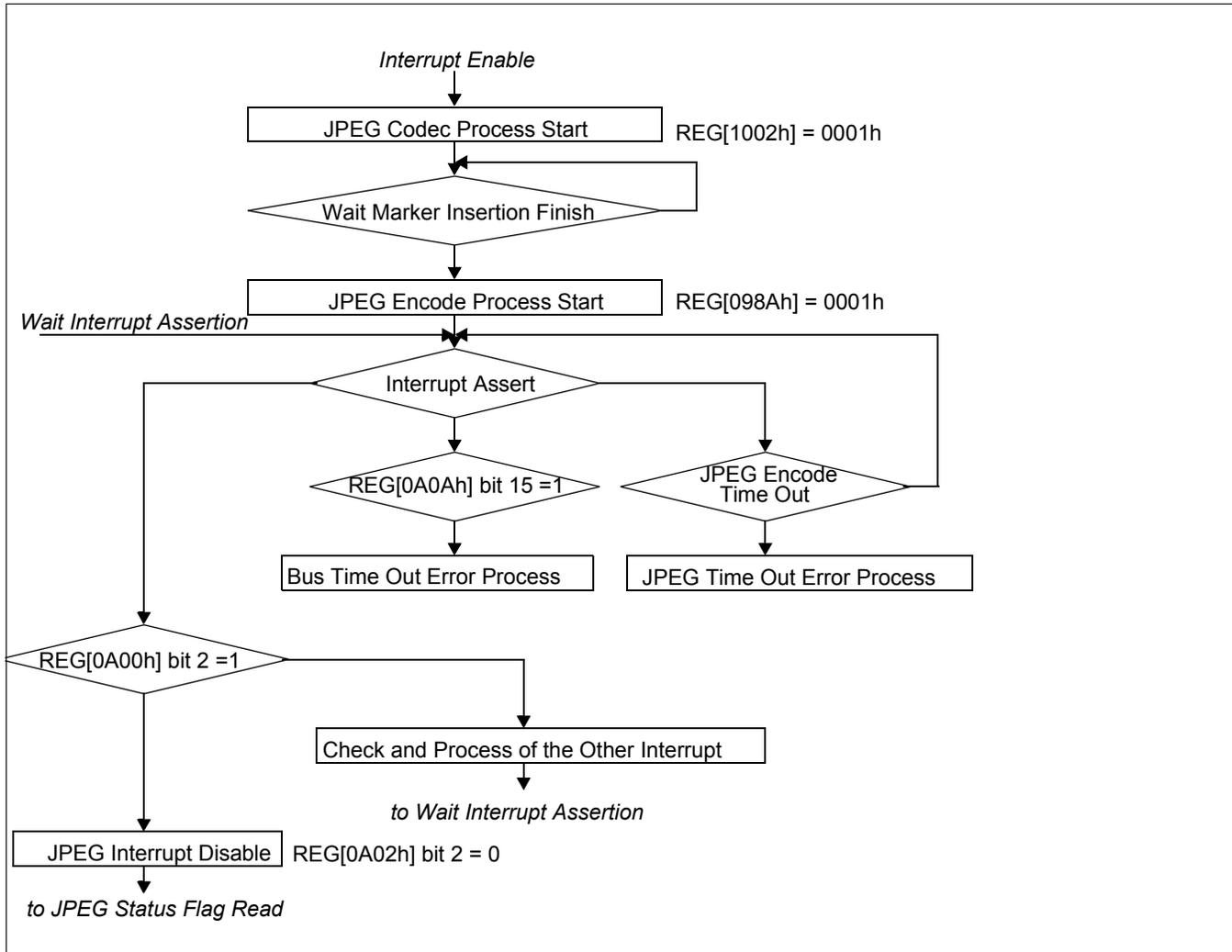
Figure 19-3: JPEG Encoding Process (2 of 4)
