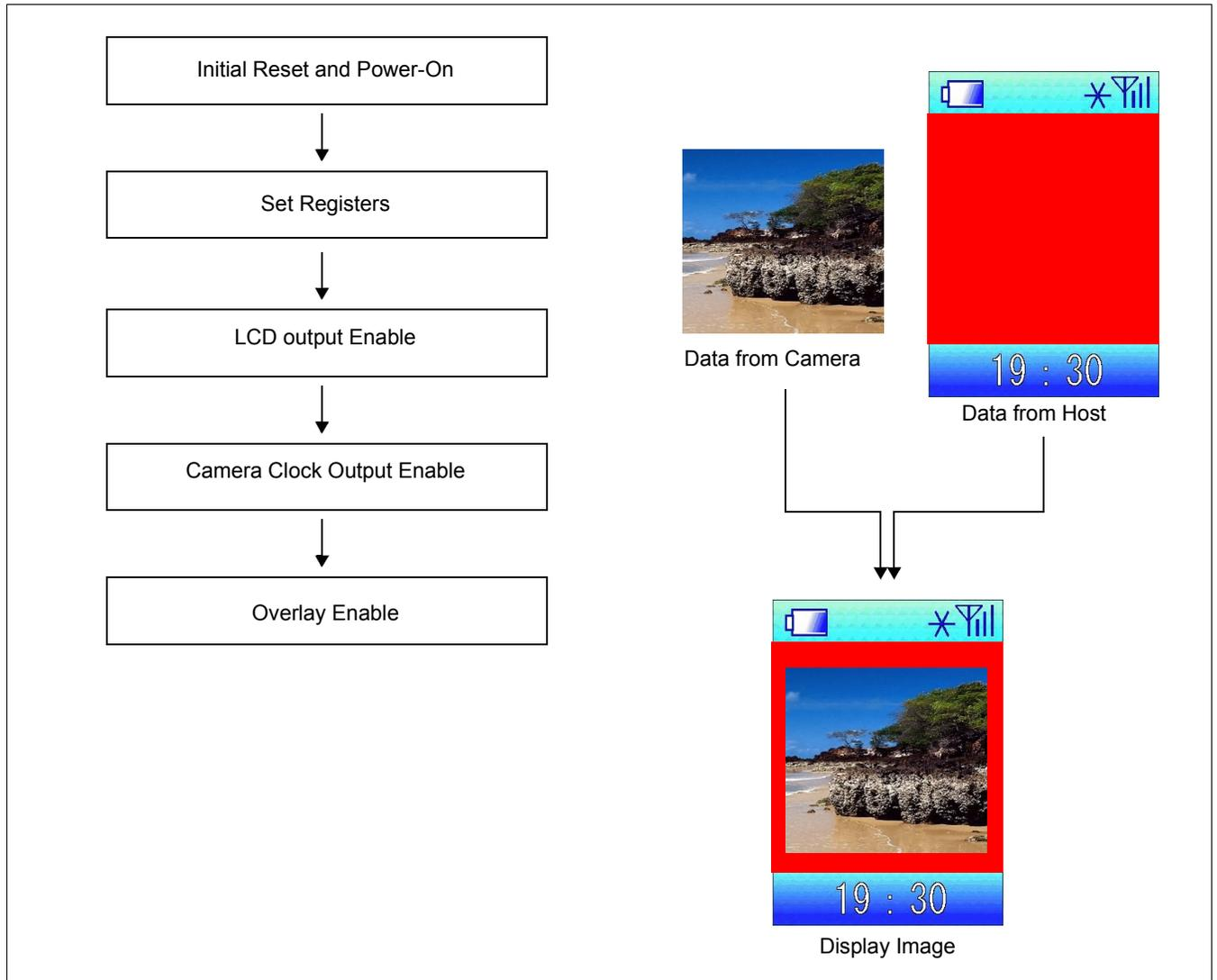
Figure 18-2: Display Image Data from the Camera Interface
