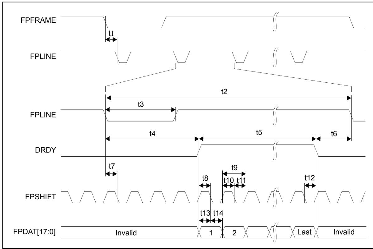
Figure 7-31: Generic RGB Type Interface Panel Horizontal Timing
