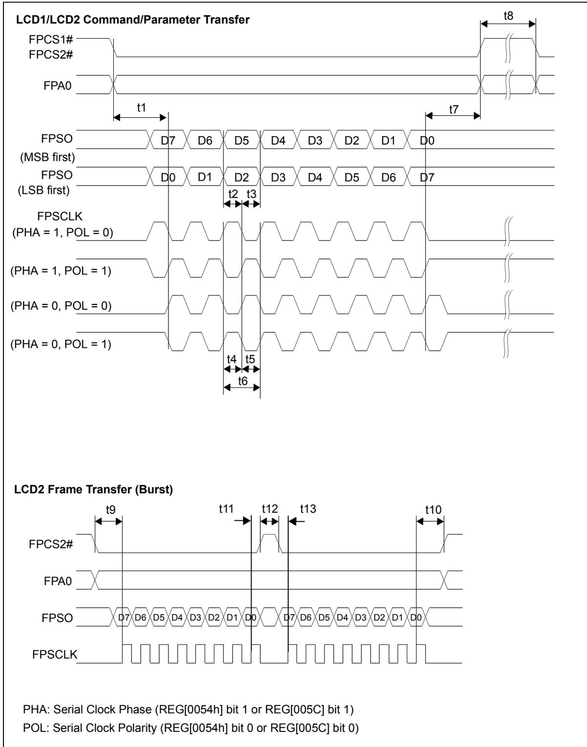
Figure 7-33: LCD1 ND-TFD, LCD2 8-Bit Serial Interface Timing
