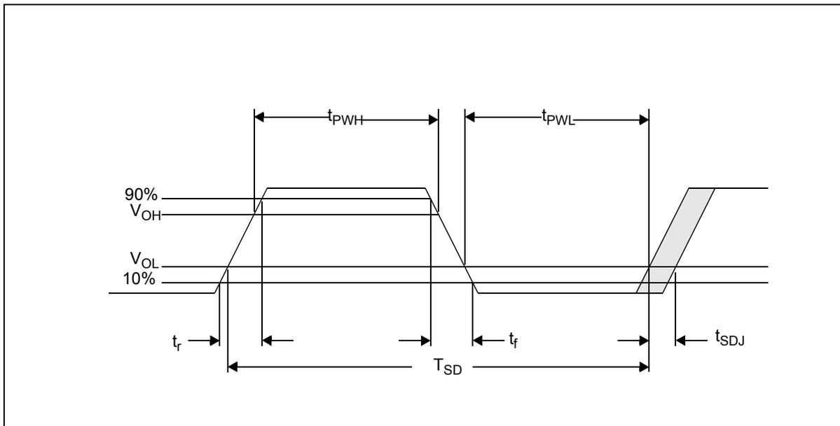
Figure 7-45: SD Memory Card Clock Output Timing
