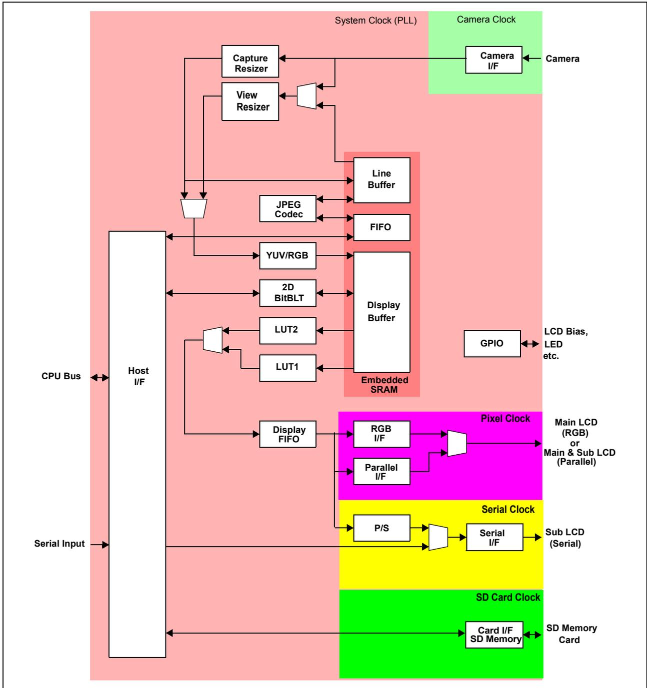
Figure 4-1: SID13717 Block Diagram
