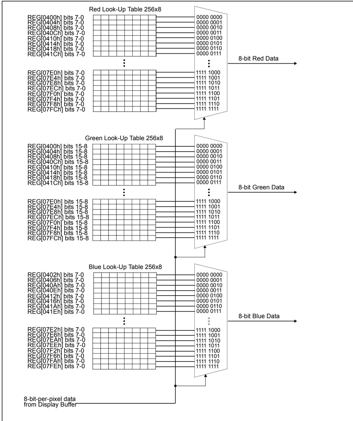
Figure 12-1: LUT1 (Main Window) for 8 Bpp Architecture
