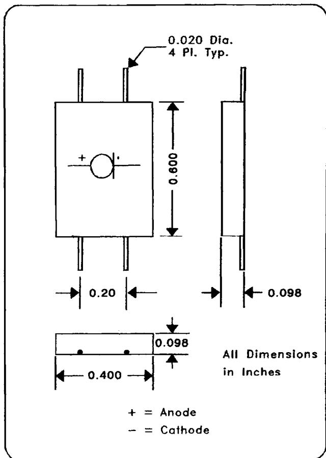
Glass Diodes encapsulated in liquid polymer case.
