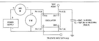
NOTE A: C<sub>L</sub> includes probe and fixture capacitance
