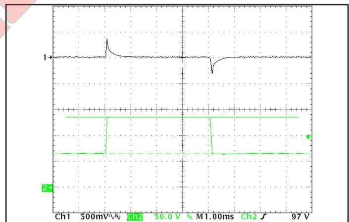
Figure 6: Output voltage response to step-change in input voltage (1000 V/ms). Load cap: 1 μF ceramic and 15 μF tantalum capacitors. Ch 1: V<sub>out</sub>, Ch 2: V<sub>in</sub>.
