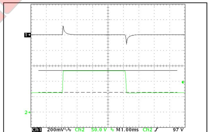
Figure 6: Output voltage response to step-change in input voltage (1000 V/μs). Load cap: 1 μF ceramic and 15 μF tantalum capacitors. Ch 1: V<sub>out</sub>, Ch 2: V<sub>in</sub>.
