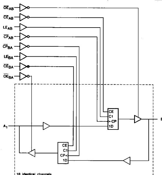
Fig.4 Logic diagram (one section)
