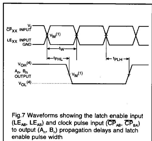
Fig.7 Waveforms showing the latch enable input ( $\overline{LE}_{AB}, \overline{LE}_{BA}$ ) and clock pulse input ( $\overline{CP}_{AB}, \overline{CP}_{BA}$ ) to output ( $A_n, B_n$ ) propagation delays and latch enable pulse width
