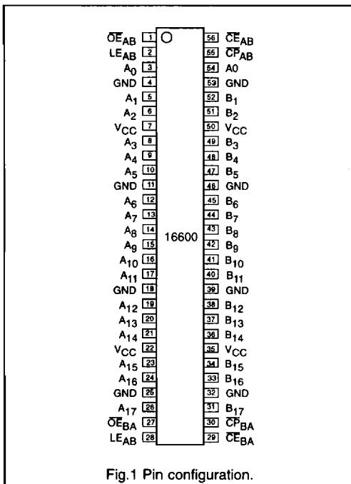
Fig.1 Pin configuration.
