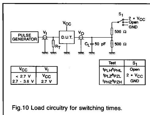
Fig.10 Load circuitry for switching times.
