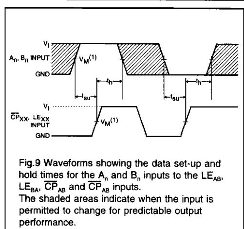
Fig.9 Waveforms showing the data set-up and hold times for the  $A_n$  and  $B_n$  inputs to the  $\overline{LE}_{AB}, \overline{LE}_{BA}, \overline{CP}_{AB}$  and  $\overline{CP}_{BA}$  inputs.
