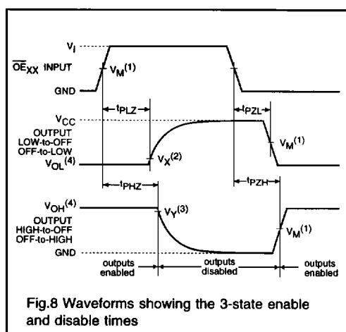
Fig.8 Waveforms showing the 3-state enable and disable times
