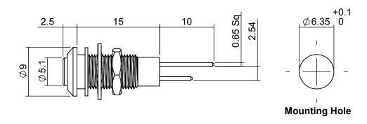
Dimensions in mm (typical) Not to scale Anode termination denoted by red indicator Mounting hole to be clean and burr free
