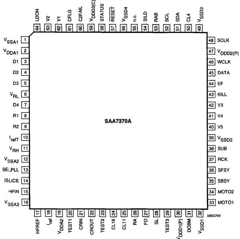
Fig.2 Pin configuration.
