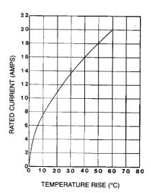
CURVES DEVELOPED USING SERIES 41 CONNECTORS AND 16 AWG (1,5  $\mathrm{MM}^2$ ) SIZE WIRE. ALL CONTACTS UNDER LOAD.
