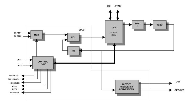
Figure 1. - The functional block diagram of SY0006
