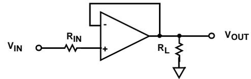
FIGURE 38. INPUT CURRENT LIMITING
