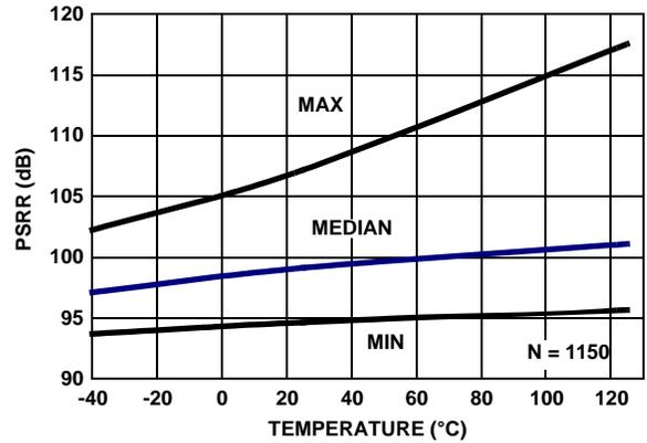
FIGURE 33. PSRR vs TEMPERATURE,  $V_+$ ,  $V_- = \pm 1.2V$  TO  $\pm 2.75V$
