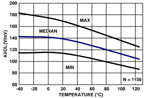
FIGURE 35. AVOL vs TEMPERATURE,  $V_+$ ,  $V_- = \pm 2.5V$ ,  $V_O = -2V$  TO  $+2V$ ,  $R_L = 1k$
