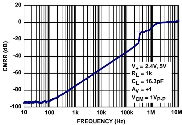
FIGURE 9. CMRR vs FREQUENCY;  $V_+ = 2.4V$  AND  $5V$
