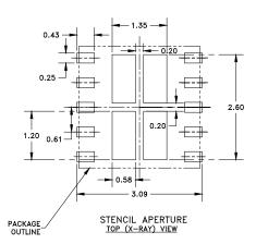
Figure 15: Recommended PCB Layout Information
