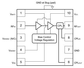
Figure 1: Block Diagram
