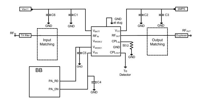
Figure 12: Typical Application Circuit
