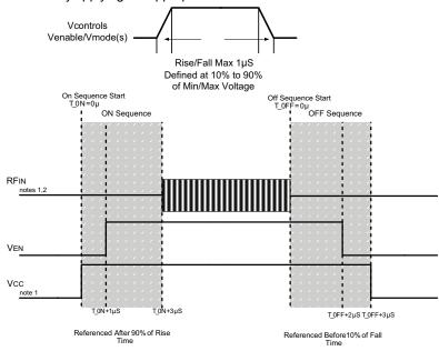
Figure 9: Recommended ON/OFF Timing Sequence
