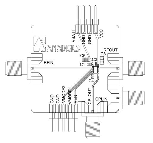
Figure 11: Evaluation Board Layout
