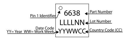
Figure 14: Branding Specification Package
