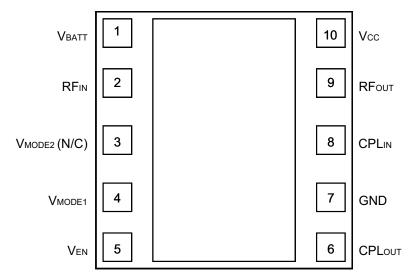
Figure 2: Pinout (X-ray Top View)
