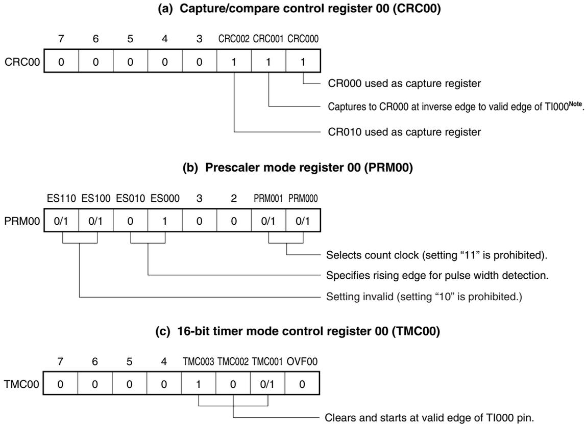
**Note** If the valid edge of TI000 pin is specified to be both the rising and falling edges, 16-bit timer capture/compare register 000 (CR000) cannot perform the capture operation.
