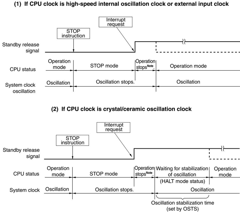
**Note** The operation stop time is 17  $\mu s$  (MIN.), 34  $\mu s$  (TYP.), and 67  $\mu s$  (MAX.).
