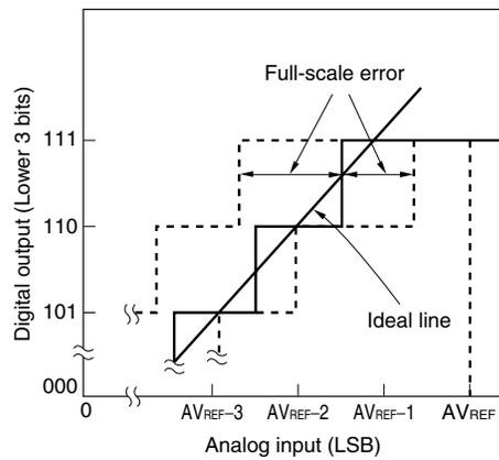
**Figure 10-17. Integral Linearity Error**
