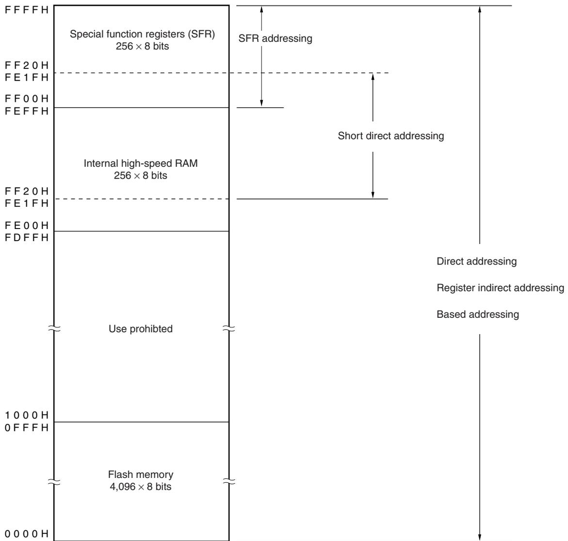
Figure 3-4. Data Memory Addressing ( $\mu$ PD78F9234)
