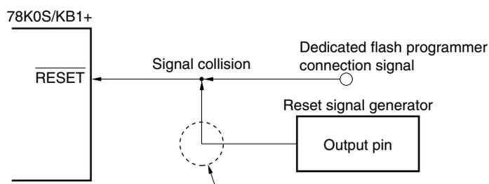
In the flash memory programming mode, the signal output by the reset signal generator collides with the signal output by the dedicated flash programmer. Therefore, isolate the signal of the reset signal generator.
