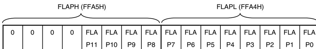
**Caution** Be sure to clear bits 4 to 7 of FLAPH and FLAPHC to 0 before executing the self programming command. If the value of these bits is 1 when executing the self programming command.
