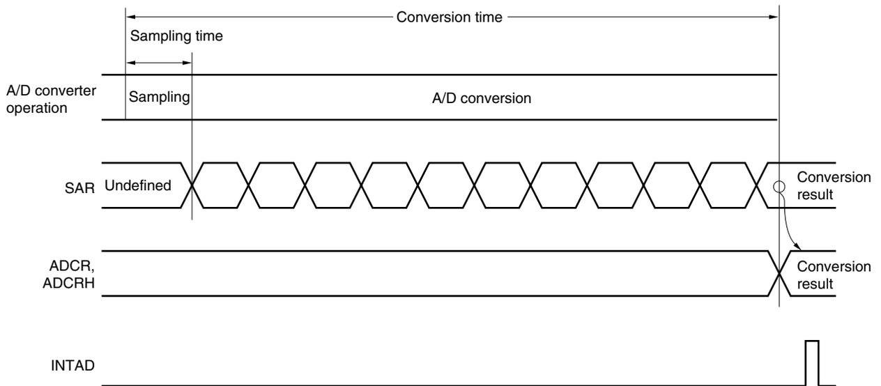
A/D conversion operations are performed continuously until bit 7 (ADCS) of the A/D converter mode register (ADM) is reset (0) by software.
