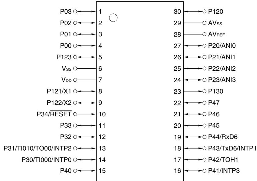
**Caution** Connect the AV<sub>ss</sub> pin to V<sub>ss</sub>.
