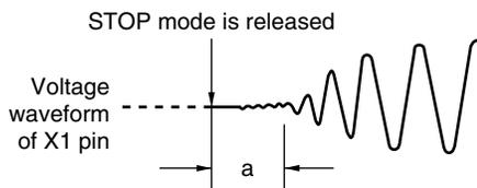
**Caution 3. The oscillation stabilization time that elapses on power application or after release of reset is selected by the option byte. For details, refer to CHAPTER 18 OPTION BYTE.**
