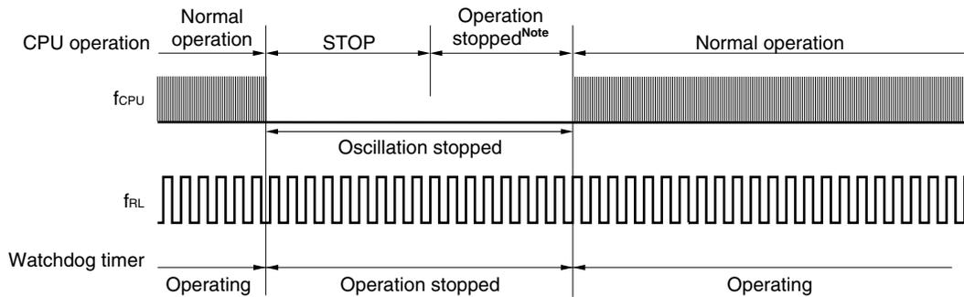
**Note** The operation stop time is  $17 \mu\text{s}$  (MIN.),  $34 \mu\text{s}$  (TYP.), and  $67 \mu\text{s}$  (MAX.).
