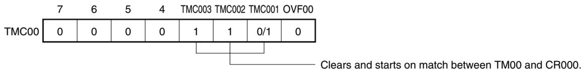
**Remark** 0/1: Setting 0 or 1 allows another function to be used simultaneously with the external event counter. See the description of the respective control registers for details.
