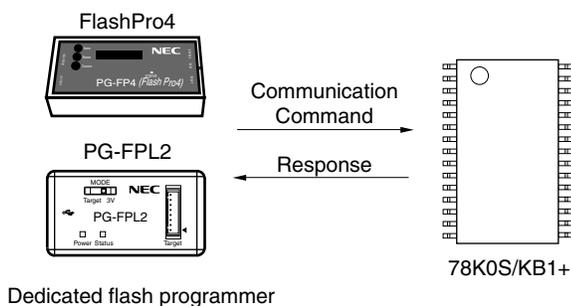
Communication commands are listed in the table below. All these communication commands are issued from the programmer and the 78K0S/KB1+ perform processing corresponding to the respective communication commands.
