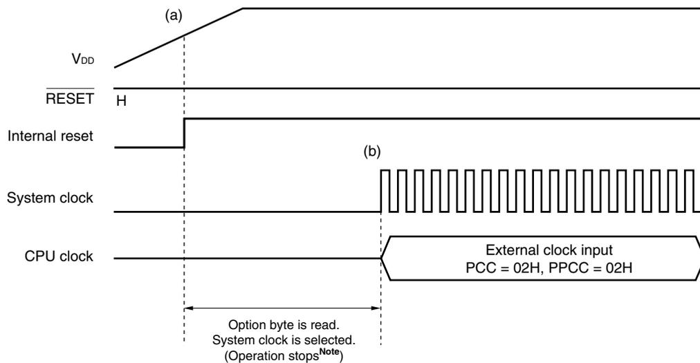
**Note** Operation stop time is 277  $\mu$ s (MIN.), 544  $\mu$ s (TYP.), and 1.075 ms (MAX.).
