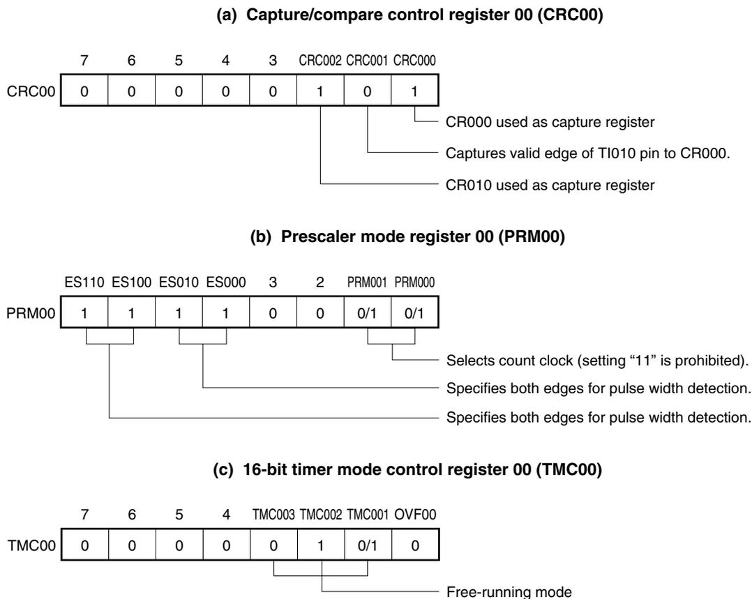
**Remark** 0/1: Setting 0 or 1 allows another function to be used simultaneously with pulse width measurement. See the description of the respective control registers for details.
