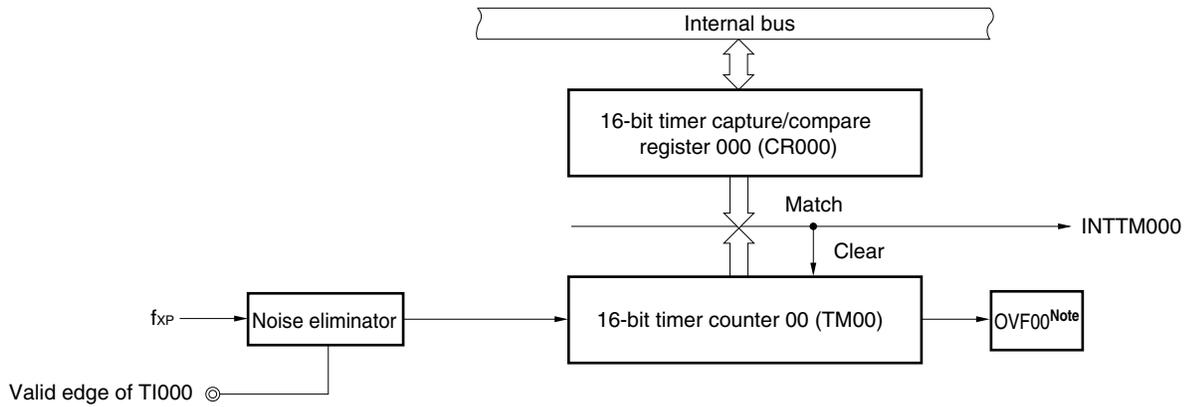
**Note** OVF00 is 1 only when 16-bit timer capture/compare register 000 (CR000) is set to FFFFH.
