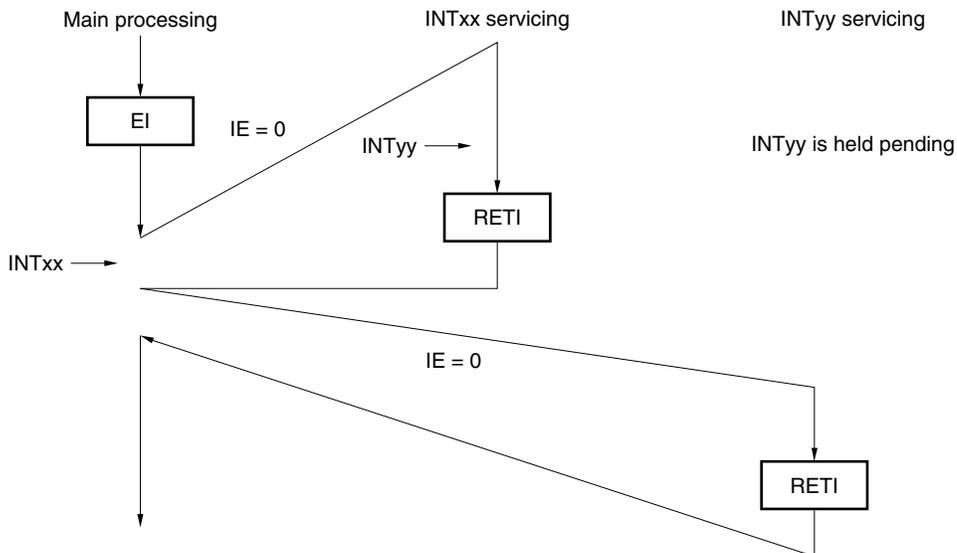
Because interrupts are not enabled in interrupt INTxx servicing (the EI instruction is not issued), interrupt request INTyy is not acknowledged, and multiple interrupts are not generated. The INTyy request is held pending and acknowledged after the INTxx servicing is performed.
