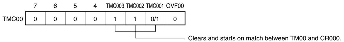
**Remark** 0/1: Setting 0 or 1 allows another function to be used simultaneously with the interval timer. See the description of the respective control registers for details.
