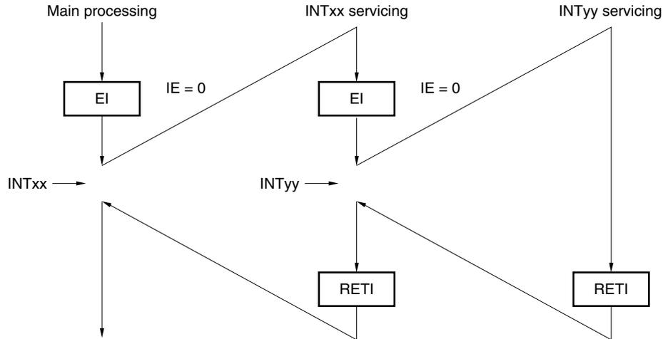
During interrupt INTxx servicing, interrupt request INTyy is acknowledged, and multiple interrupts are generated. Before each interrupt request acknowledgement, the EI instruction is issued, the interrupt mask is released, and the interrupt request acknowledgement enable state is set.
