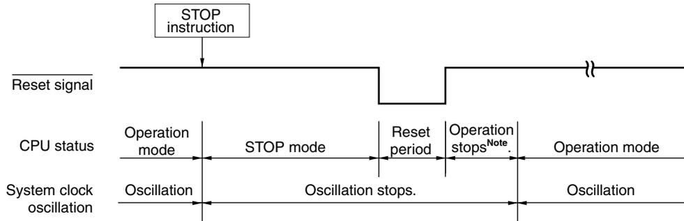
**Note** Operation is stopped (277  $\mu$ s (MIN.), 544  $\mu$ s (TYP.), 1.075 ms (MAX.)) because the option byte is referenced.
