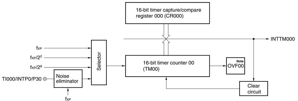
**Note** OVF00 is set to 1 only when 16-bit timer capture/compare register 00 (CR000) is set to FFFFH.
