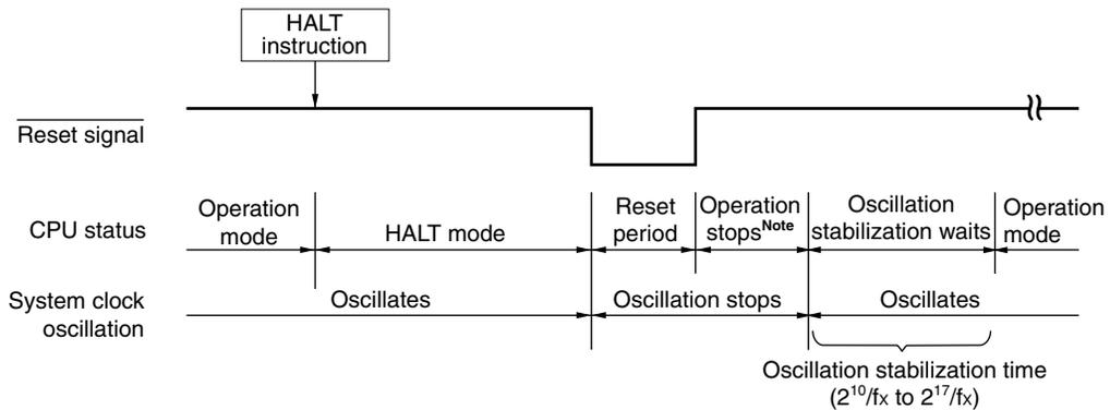
**Note** Operation is stopped (276  $\mu$ s (MIN.), 544  $\mu$ s (TYP.), 1.074 ms (MAX.)) because the option byte is referenced.
