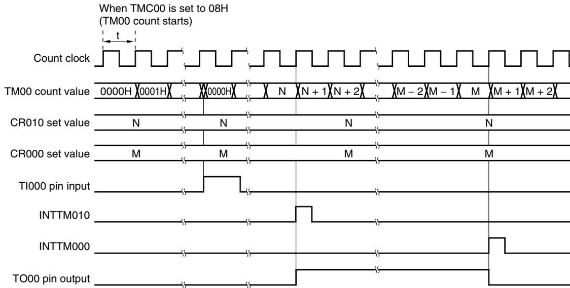
**Caution** 16-bit timer counter 00 starts operating as soon as a value other than 0, 0 (operation stop mode) is set to the TMC003 and TMC002 bits.
