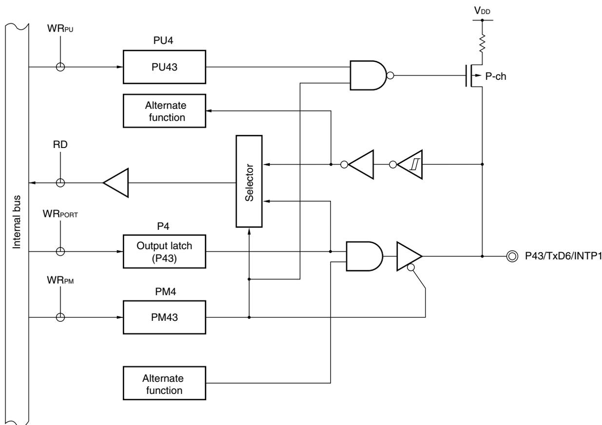
PU4: Pull-up resistor option register 4
