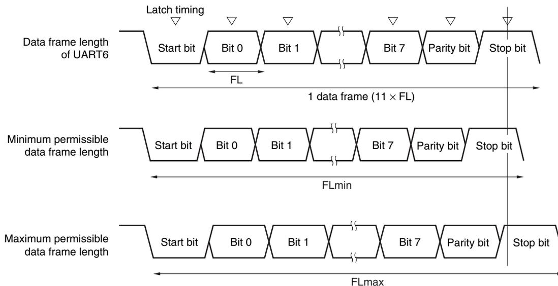
As shown in Figure 11-25, the latch timing of the receive data is determined by the counter set by baud rate generator control register 6 (BRGC6) after the start bit has been detected. If the last data (stop bit) meets this latch timing, the data can be correctly received.
