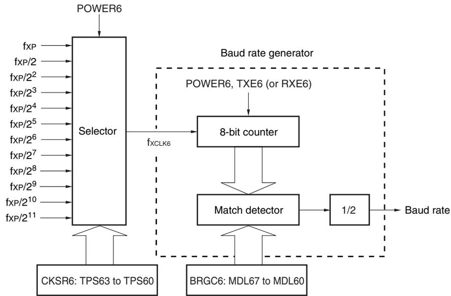
**Remark** POWER6: Bit 7 of asynchronous serial interface operation mode register 6 (ASIM6)
