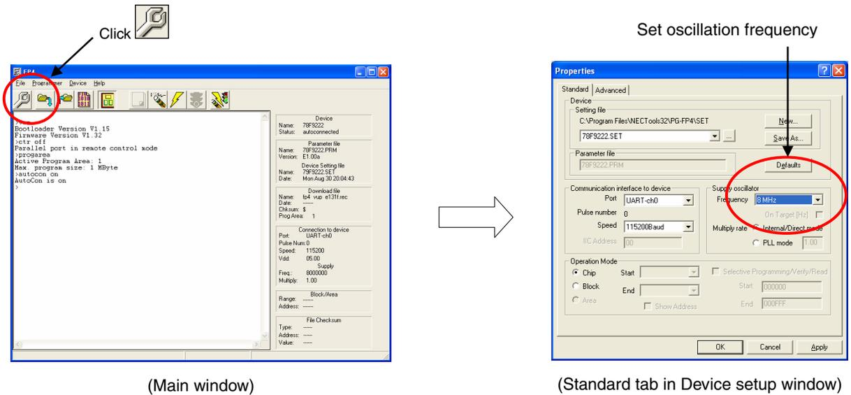
Table 19-5. Oscillation Frequency and PG-FP4 GUI Software Setting Value Example
