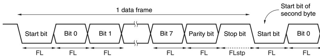
Where the 1-bit data length is FL, the stop bit length is FLstp, and base clock frequency is  $f_{\text{CLK6}}$ , the following expression is satisfied.
