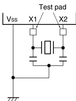
**Table 19-4. Clock to Be Used and Mounting of Test Pads**
