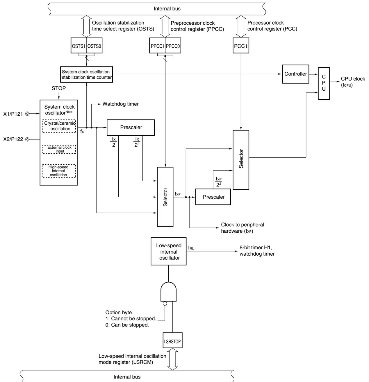
**Note** Select the high-speed internal oscillator, crystal/ceramic oscillator, or external clock input as the system clock source by using the option byte.
