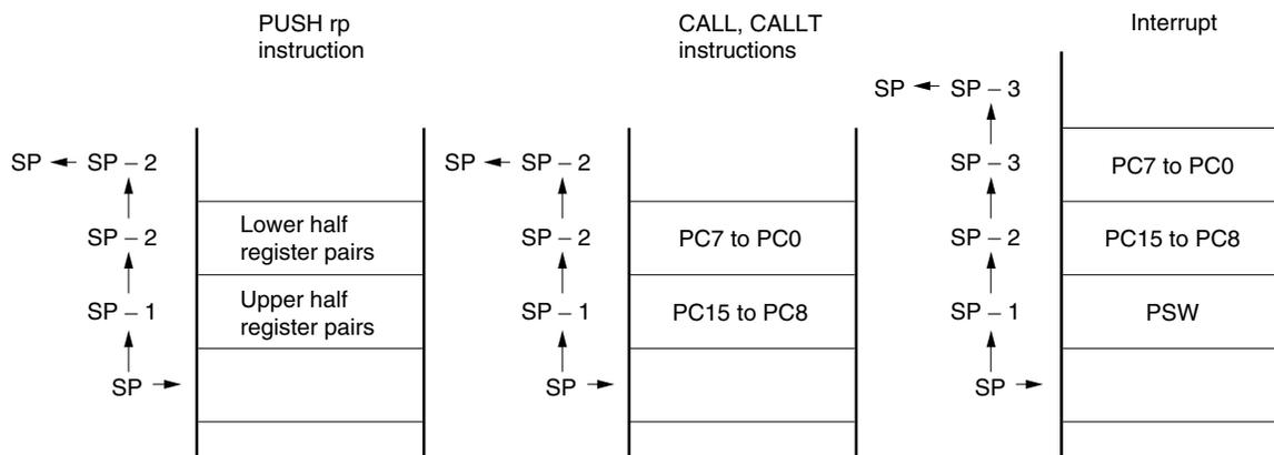
Figure 3-9. Data to Be Restored from Stack Memory
