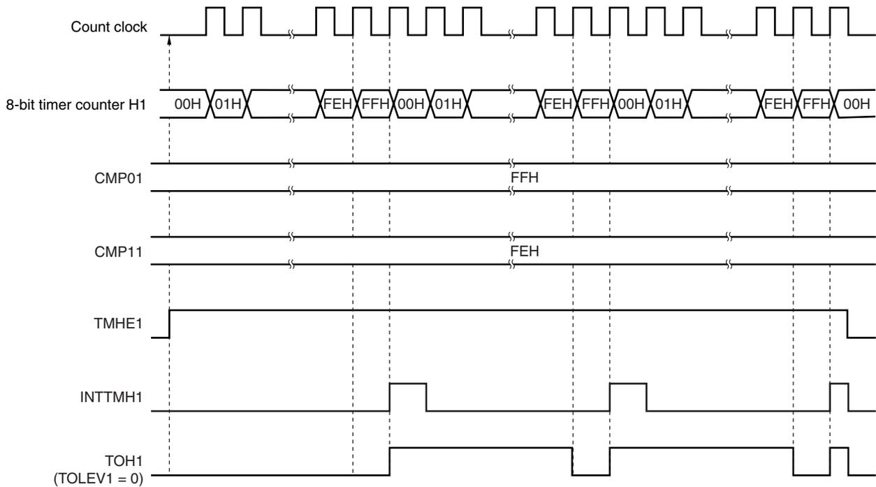
Figure 8-9. Operation Timing in PWM Output Mode (3/4)
