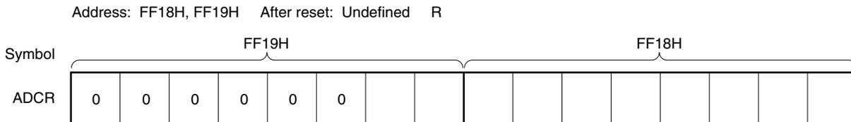
**Caution** When writing to the A/D converter mode register (ADM) and analog input channel specification register (ADS), the contents of ADCR may become undefined. Read the conversion result following conversion completion before writing to ADM and ADS. Using timing other than the above may cause an incorrect conversion result to be read.
