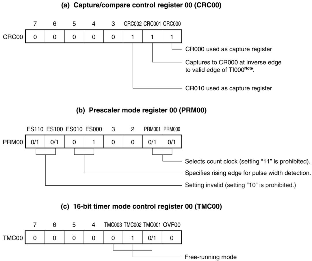
**Note** If the valid edge of TI000 pin is specified to be both the rising and falling edges, 16-bit timer capture/compare register 000 (CR000) cannot perform the capture operation. When the CRC001 bit value is 1, the TM00 count value is not captured in the CR000 register when a valid edge of the TI010 pin is detected, but the input from the TI010 pin can be used as an external interrupt source because INTTM000 is generated at that timing.
