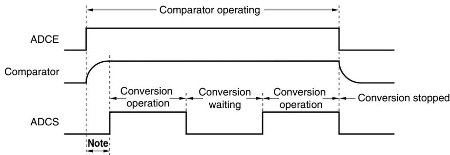
**Note** The time from the rising of the ADCE bit to the rising of the ADCE bit must be  $1\ \mu\text{s}$  or longer to stabilize the internal circuit.
