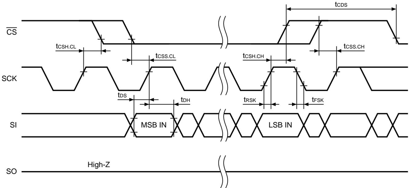
Figure 4 Serial Input Timing
