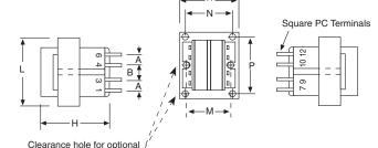
The RL-2252 Series International Power Transformers are designed to meet UL, VDE, IEC, CSA requirements. Available in rating of 2.5 through 50VA. Designed to UL1585 Class 2 with all primaries thermally protected for your safety. PC Board mount with all advantages of RL-2250 International Series. Hipot tested at 4000VRMS. Manufactured to Class B (130°) Insulation.
