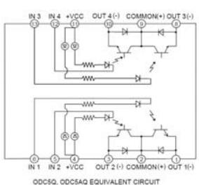
DC INDUCTIVE LOADS MUST BE DIODE SUPPRESSED
