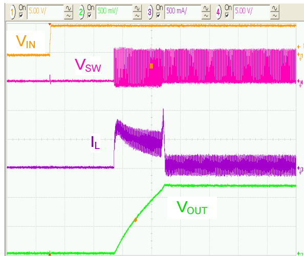
Figure 4. Startup with 100mA Resistive Load
