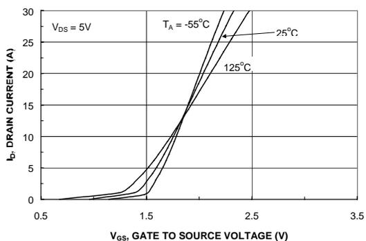
Figure 5. Transfer Characteristics.
