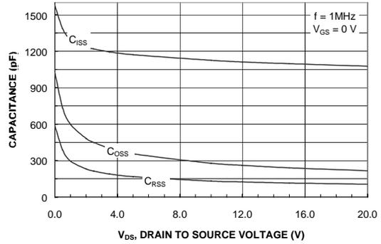
Figure 8. Capacitance Characteristics.
