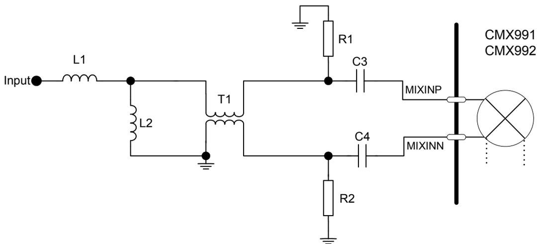
Figure 6 Example External Components – Receive 1<sup>st</sup> Mixer Input
