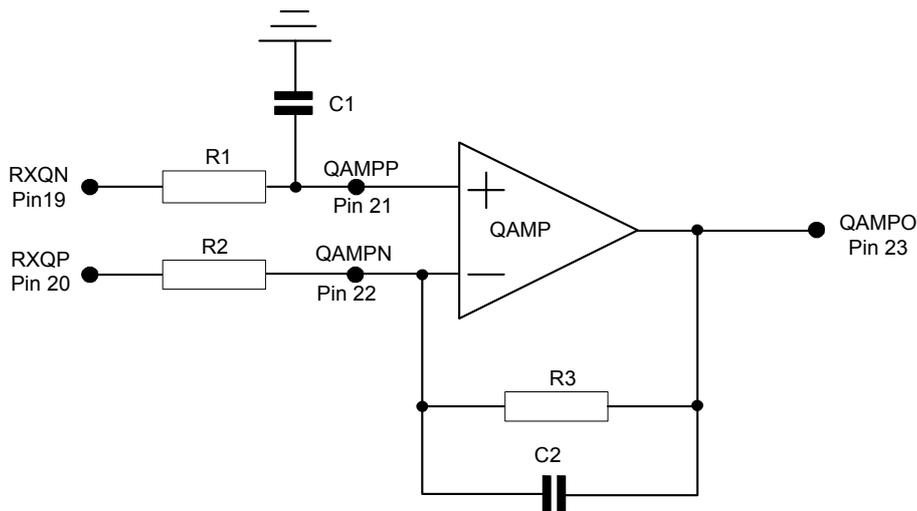
**Figure 8 Example External Components – Receive I/Q Output**
