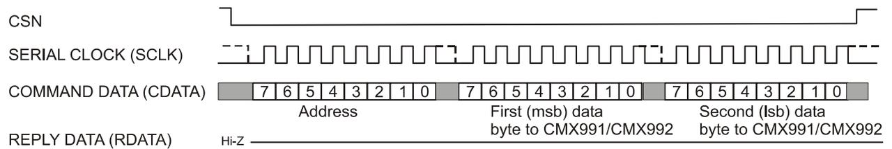
**d) One Address byte from  $\mu$ C and one Reply byte from CMX991/CMX992**
