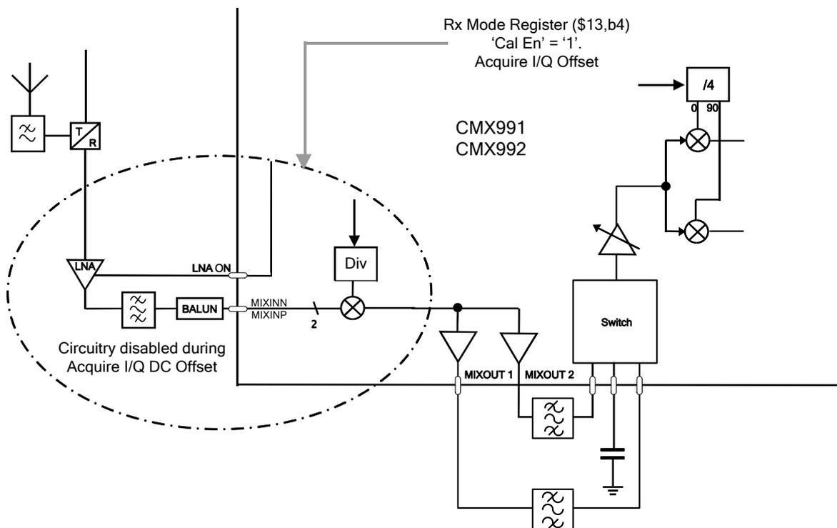
Figure 15 DC Offset Calibration Mode
