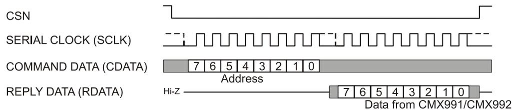
**e) One Address byte from  $\mu$ C and 2 Reply bytes from CMX991/CMX992**
