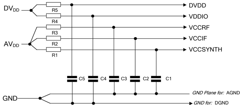
**Figure 5 Recommended Power Supply Connections and Decoupling**
