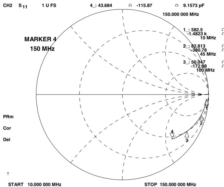
**Figure 23 IFIP1 Input Impedance at 0dB attenuation**
