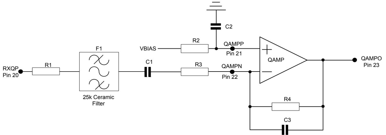
**Figure 9 Example External Components – Receive Low IF Output**
