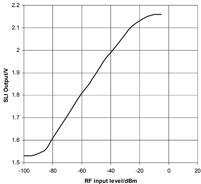
**Figure 25 Typical SLI Performance in an Application Circuit (EV9920B)**
