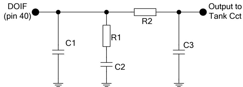
**Figure 14 Example External Components – IF LO Loop Filter**
