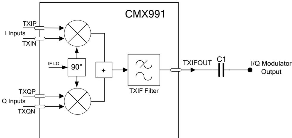
Figure 11 Example External Components – I/Q Modulator Output
