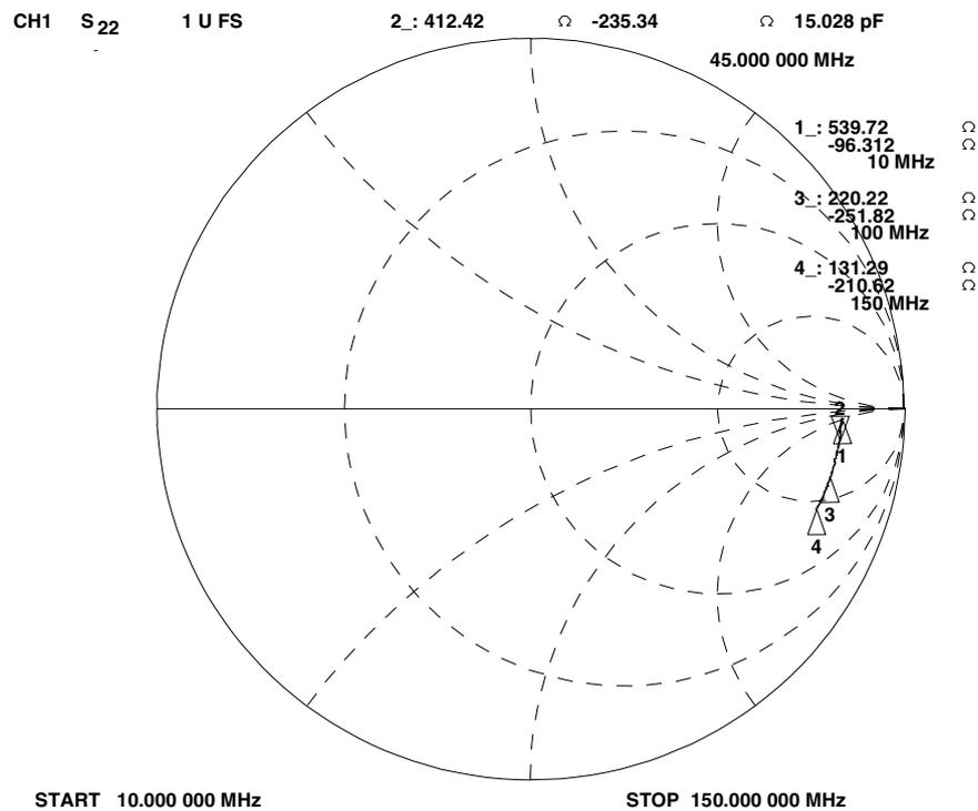
Figure 22 MIXOUT1 Port Impedance (unmatched)
