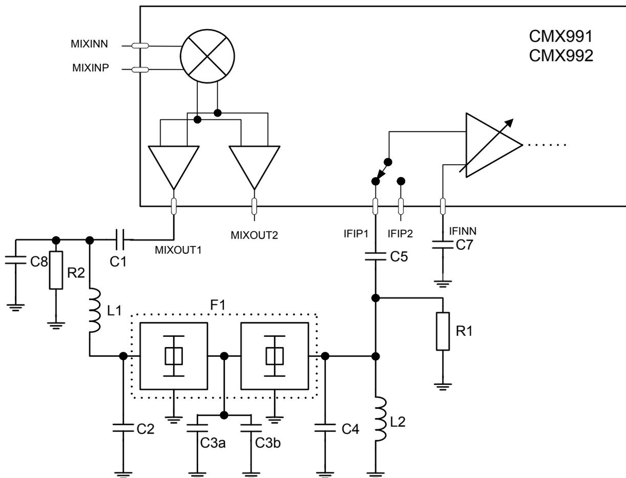
Figure 7 Example External Components – Receive 1<sup>st</sup> IF Section
