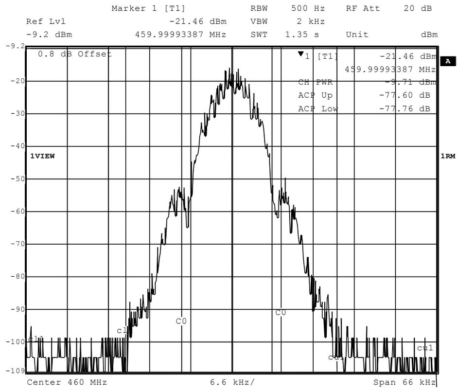
**Figure 28 Tx Output with 9.6kbps GMSK from an EV9100
