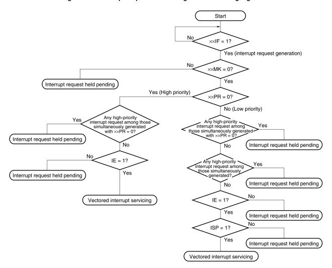
Figure 19-7. Interrupt Request Acknowledgement Processing Algorithm
