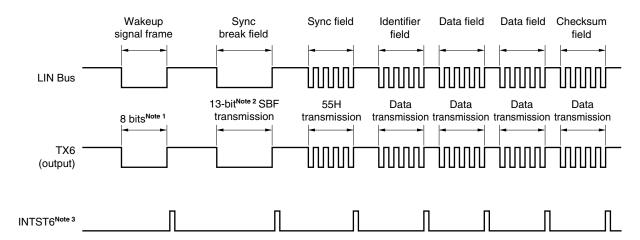
Figure 14-1. LIN Transmission Operation
