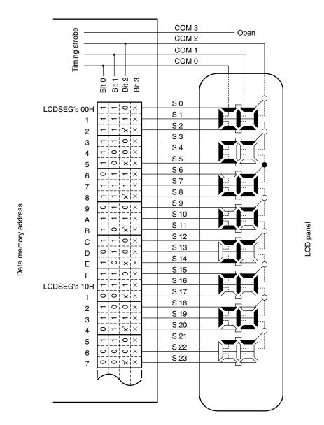
Figure 17-22. Example of Connecting Three-Time-Slice LCD Panel
