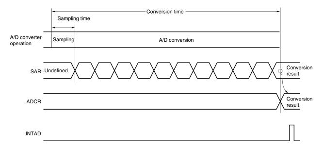
Figure 12-11. Basic Operation of A/D Converter
