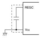
Caution Keep the wiring length as short as possible in the area enclosed by the broken lines in the above figures.
