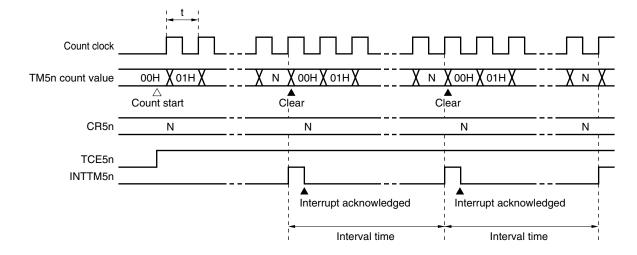
**Remark** Interval time =  $(N + 1) \times t$  N = 01H to FFHn = 0, 1
