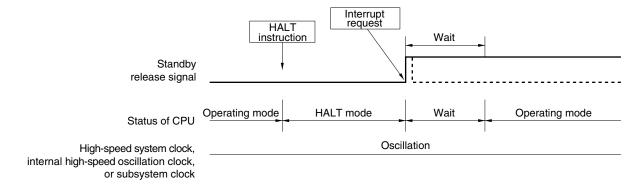
**Remarks 1.** The broken lines indicate the case when the interrupt request which has released the standby mode is acknowledged.
