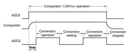
Figure 12-4. Timing Chart When Comparator Is Used
