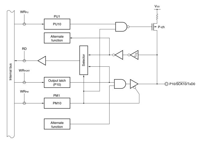
Figure 4-4. Block Diagram of P10
