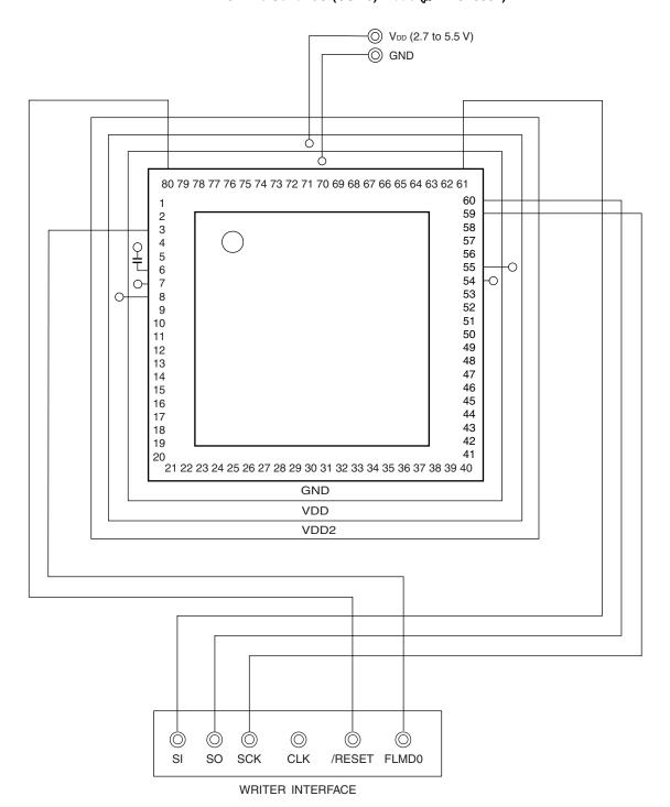
Figure 26-5. Example of Wiring Adapter for Flash Memory Writing in 3-Wire Serial I/O (CSI10) Mode ( $\mu$ PD78F038x)
