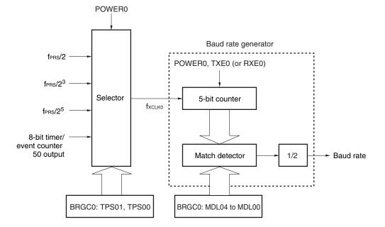
Figure 13-11. Configuration of Baud Rate Generator
