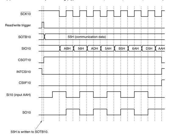
Figure 15-6. Timing of Clock/Data Phase
