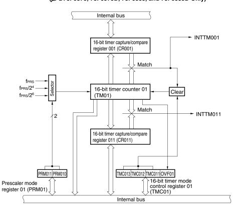
Figure 6-2. Block Diagram of 16-Bit Timer/Event Counter 01 (μPD78F0375, 78F0375D, 78F0385, and 78F0385D Only)
