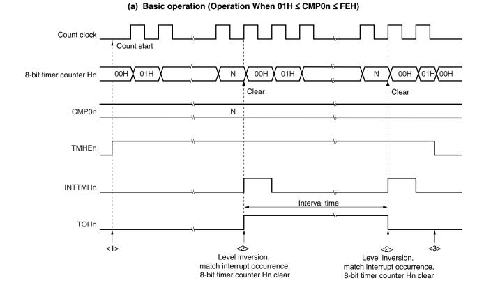
Figure 8-10. Timing of Interval Timer/Square-Wave Output Operation (1/2)
