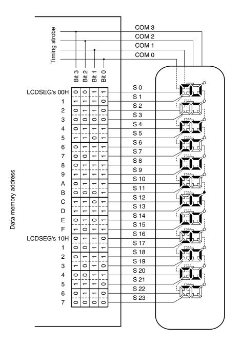
Figure 17-26. Example of Connecting Four-Time-Slice LCD Panel
