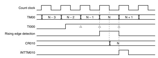
Figure 6-21. CR010 Capture Operation with Rising Edge Specified
