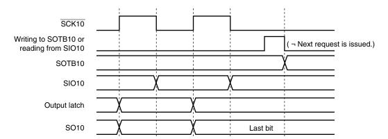
Figure 15-8. Output Value of SO10 Pin (Last Bit) (2/2)
