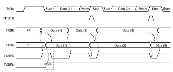
Figure 14-17. Timing of Starting Continuous Transmission
