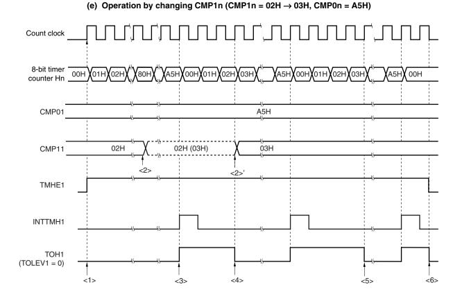
Figure 8-12. Operation Timing in PWM Output Mode (4/4)
