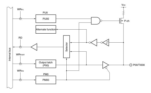
PU0: Pull-up resistor option register 0
