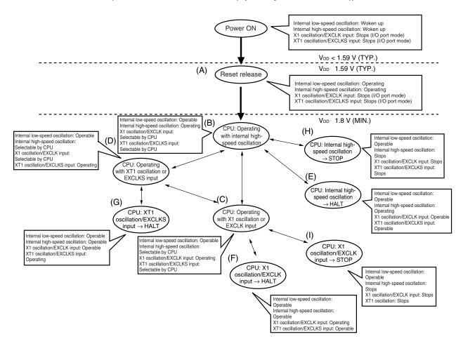
**Remark** In the 2.7 V/1.59 V POC mode (option byte: POCMODE = 1), the CPU clock status changes to (A) in the above figure when the supply voltage exceeds 2.7 V (TYP.), and to (B) after reset processing (20  $\mu$ s (TYP.)).
