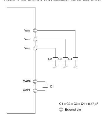
Figure 17-30. Example of Connecting Pins for LCD Driver
