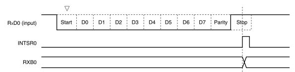
Figure 13-9. Reception Completion Interrupt Request Timing
