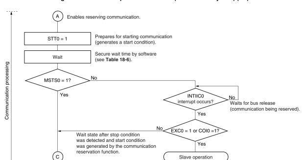
Figure 16-24. Master Operation Flowchart (Multi-Master System) (2/3)
