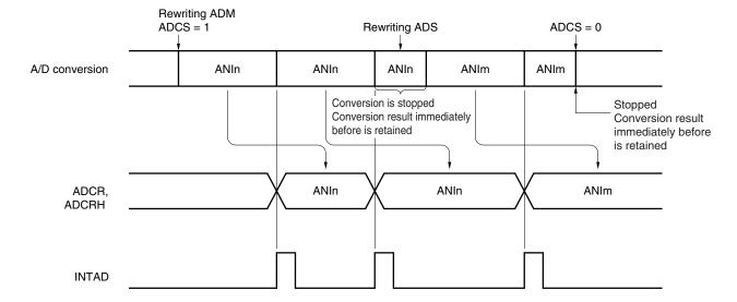
Figure 12-13. A/D Conversion Operation
