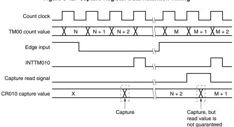
Figure 6-42. Capture Register Data Retention Timing
