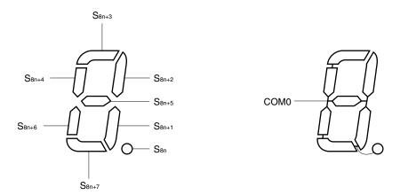
Figure 17-15. Static LCD Display Pattern and Electrode Connections
