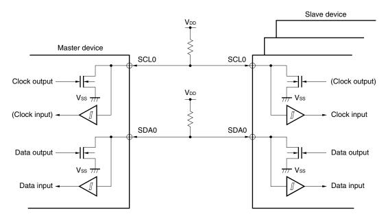
Figure 16-11. Pin Configuration Diagram
