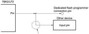
If the signal output by the 78K0/LF2 in the flash memory programming mode affects the other device, isolate the signal of the other device.
