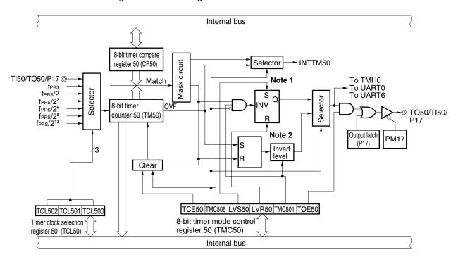
Figure 7-1. Block Diagram of 8-Bit Timer/Event Counter 50
