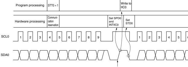
Generate by master device with bus mastership
