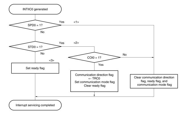
Figure 16-26. Slave Operation Flowchart (2)
