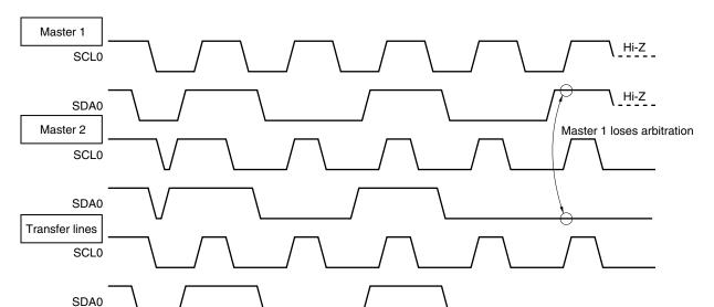
Figure 16-19. Arbitration Timing Example
