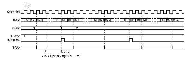
(b) CR5n value is changed from N to M after clock rising edge of FFH → Value is transferred to CR5n at second overflow.
