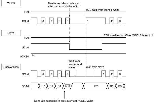
Remark ACKE0: Bit 2 of IIC control register 0 (IICC0) WREL0: Bit 5 of IIC control register 0 (IICC0)
