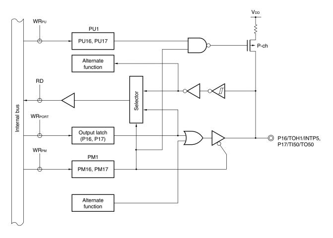
Figure 4-8. Block Diagram of P16 and P17
