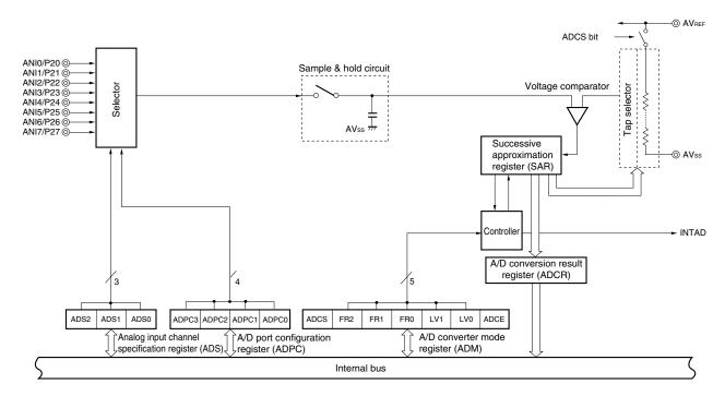
Figure 12-1. Block Diagram of A/D Converter
