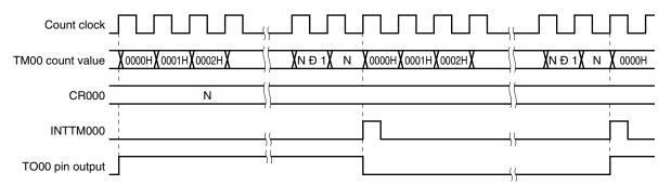
Figure 6-35. Square-Wave Output Operation Timing
