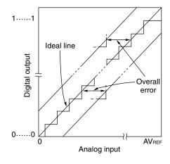
Figure 12-15. Quantization Error
