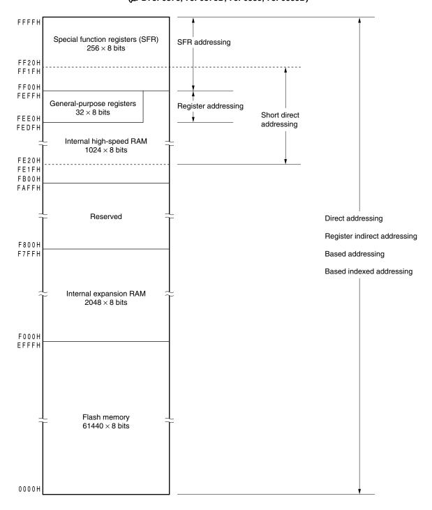
Figure 3-7. Correspondence Between Data Memory and Addressing ( $\mu$ PD78F0375, 78F0375D, 78F0385, 78F0385D)
