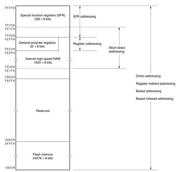
Figure 3-5. Correspondence Between Data Memory and Addressing (μPD78F0372, 78F0382)
