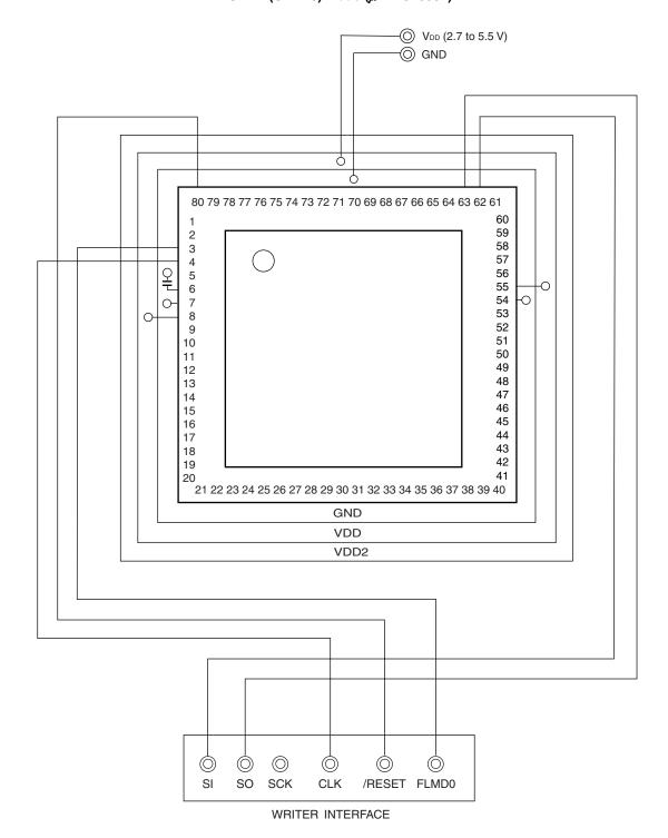
Figure 26-6. Example of Wiring Adapter for Flash Memory Writing in UART (UART6) Mode (μPD78F038x)
