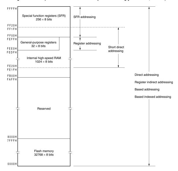
Figure 3-6. Correspondence Between Data Memory and Addressing (µPD78F0373, 78F0383)
