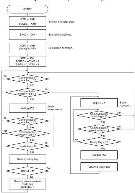
Figure 16-25. Slave Operation Flowchart (1)
