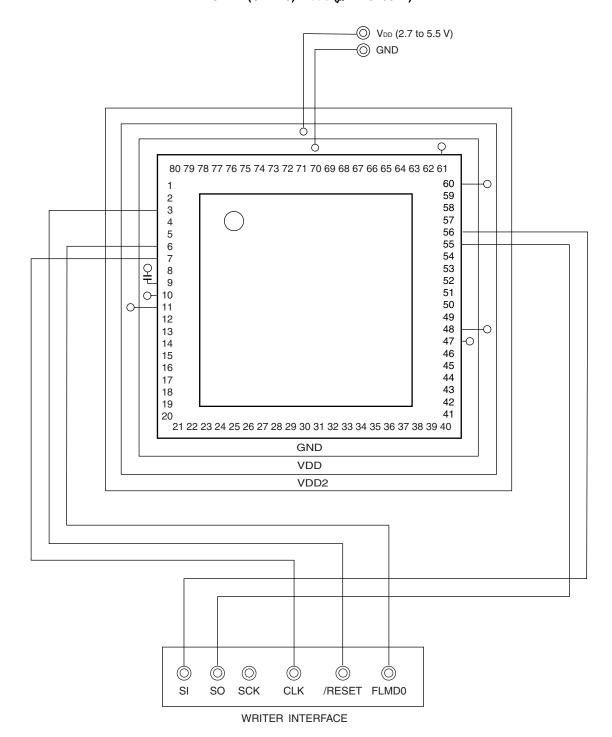
Figure 26-4. Example of Wiring Adapter for Flash Memory Writing in UART (UART6) Mode (μPD78F037x)
