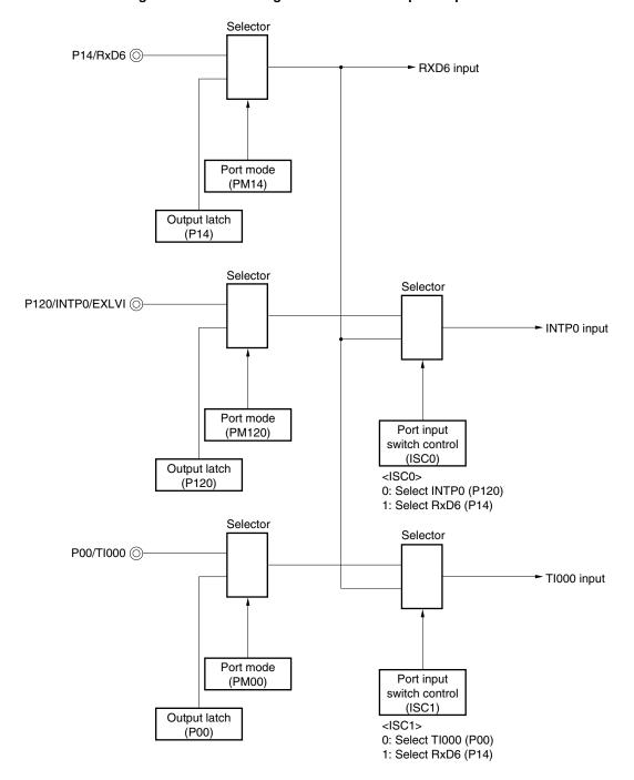
Figure 14-3. Port Configuration for LIN Reception Operation
