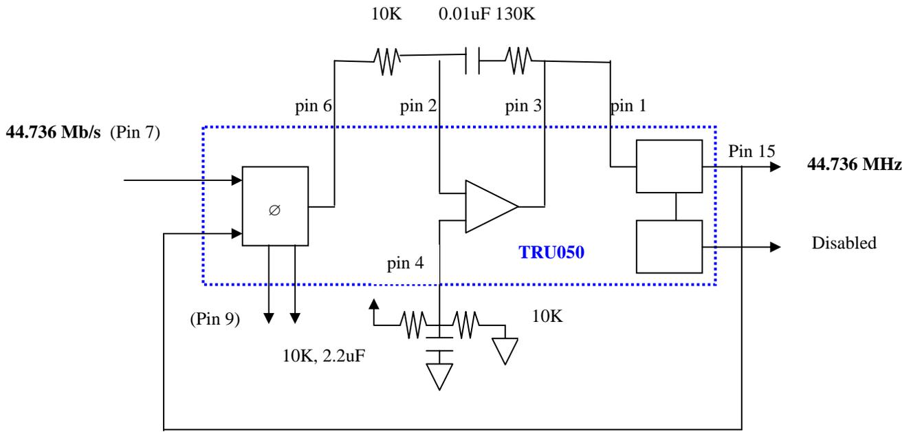
The above loop has a 4.5 kHz bandwidth.
