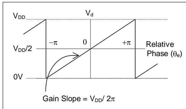
Figure 5. Open Loop Phase Detector Transfer Curve
