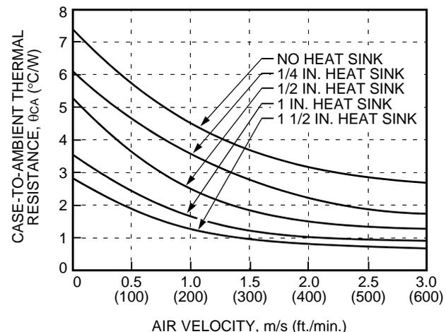
**Figure 24. Case-to-Ambient Thermal Resistance Curves; Transverse Orientation**
