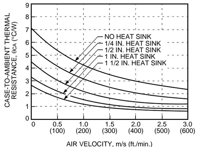
**Figure 23. Case-to-Ambient Thermal Resistance Curves; Longitudinal Orientation**
