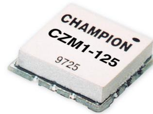
The **CZM1-125** is a fundamental mode reflection oscillator that utilizes a silicon bipolar transistor and hyper-abrupt silicon varactor diodes to create a highly linear VCO with wideband tuning characteristics. The device is useful for many wireless applications where high frequency and linear modulation is required.
