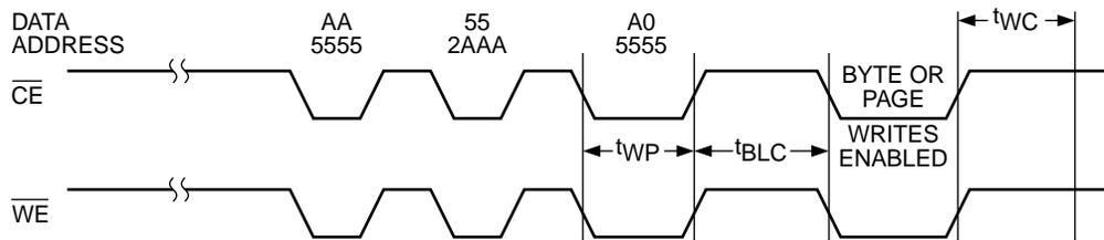
**Figure 12. Resetting Software Data Protection Timing**
