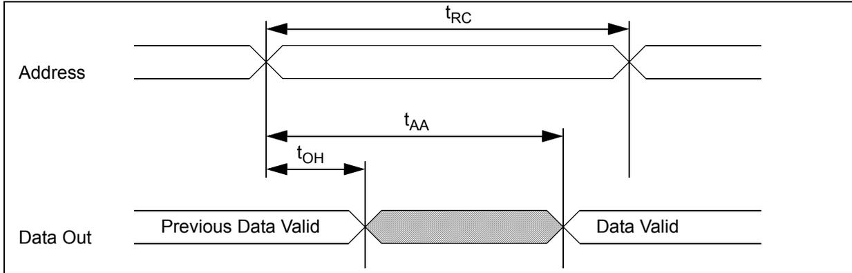
**Timing Waveform of Read Cycle ( $\overline{WE} = V_{IH}$ )**
