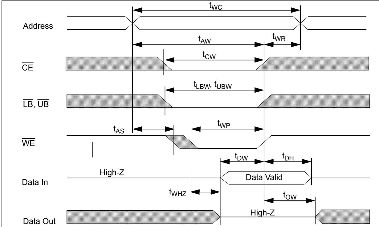
Timing Waveform of Write Cycle ( $\overline{CE}$  Control)
